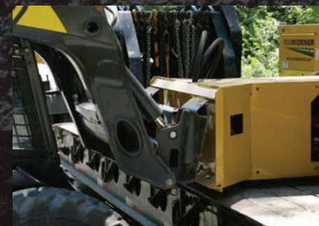
Quick connect coupler easily attaches to skid steers, loaders, and graders.
