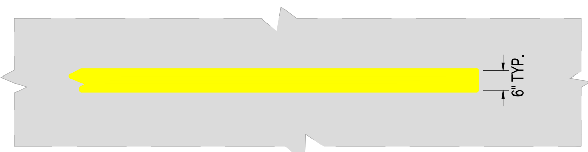
2 M-01 TAXIWAY CENTERLINE MARKING REMOVAL N.T.S.
