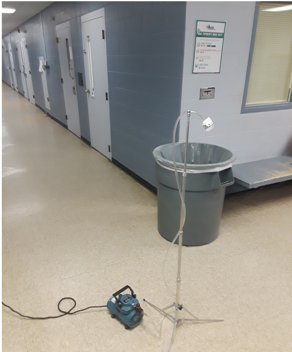
Photograph 4 Mold air sample (AIR04) collected in Booking located in the jail area.
