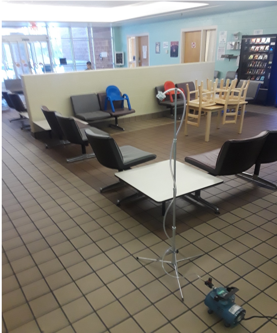
Photograph 3 Mold air sample (AIR03) collected in Lobby at main entrance.
