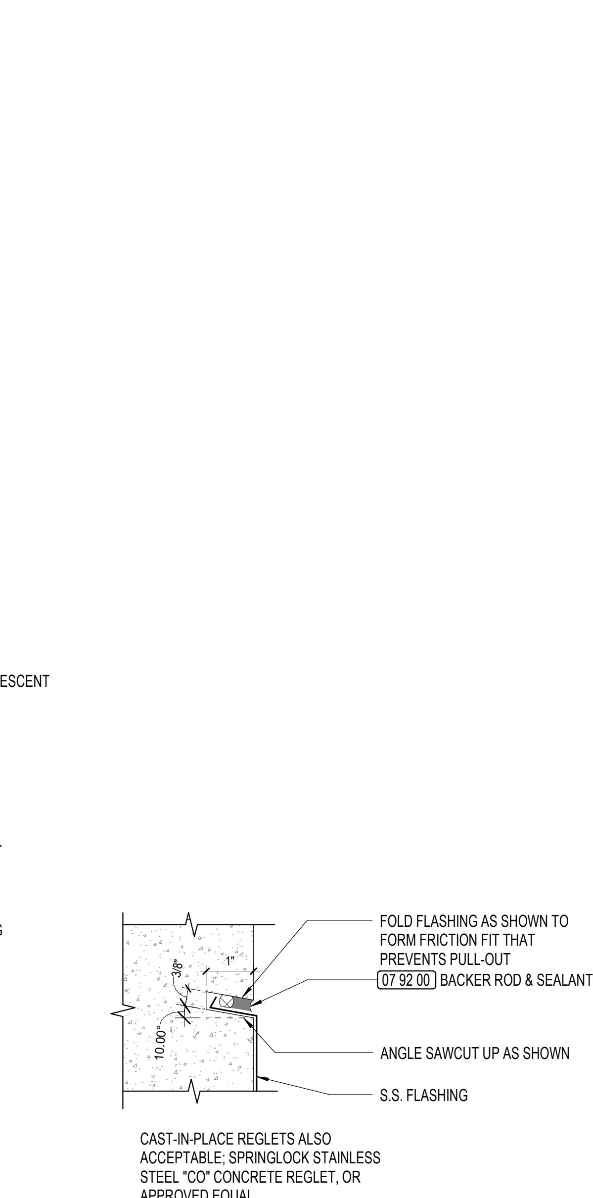
20 TYPICAL SAW-CUT REGLET SECTION 6" = 1'-0"
