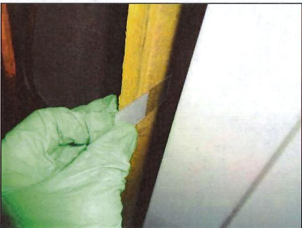
Figure (17) – City Hall HVAC Unit #2 Tape Lift Sample #CH-2 from Return Air System
