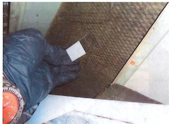
Figure (24) – #1 Tape Lift Sample from #1 HVAC Return
