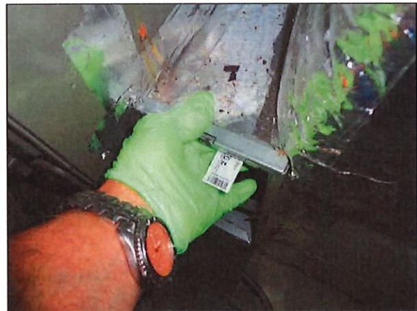
**Figure (12)** – Fire Department HVAC Unit #2 Tape Lift Sample #FD-2 from Return Air System
