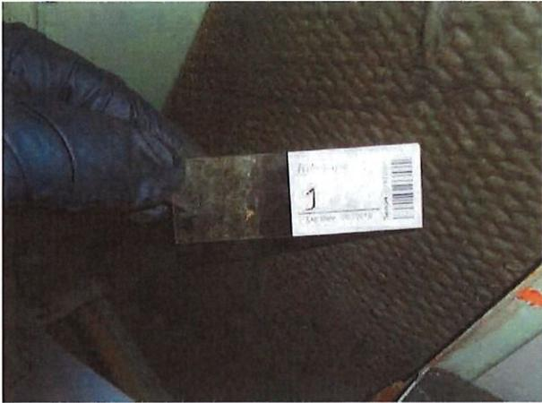
Figure (25) – #1 Tape Lift Sample from #1 HVAC Return
