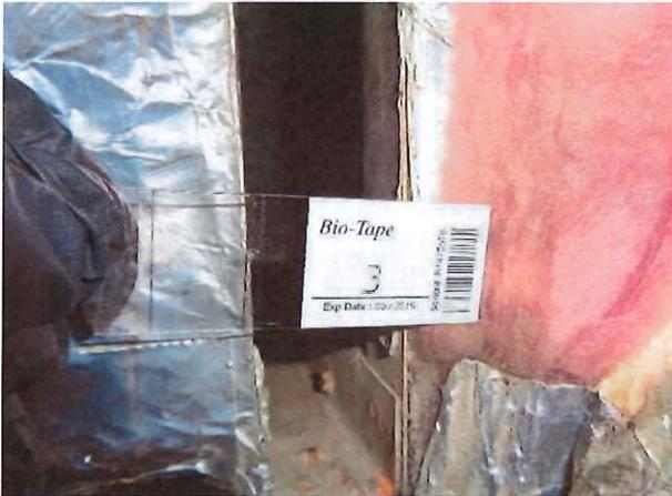
Figure (31) – #3 Tape Lift Sample from #2 HVAC System return
