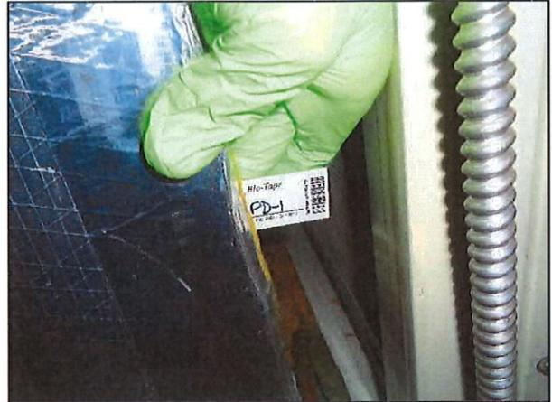
Figure (20) – Police Department HVAC Unit #1 Tape Lift Sample #PD-1 from Return Air System
