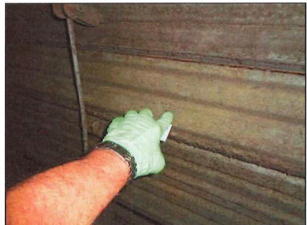
Figure (4) – Convention Center HVAC Unit #56 Tape Lift Sample #CC-1 in Return Air System
