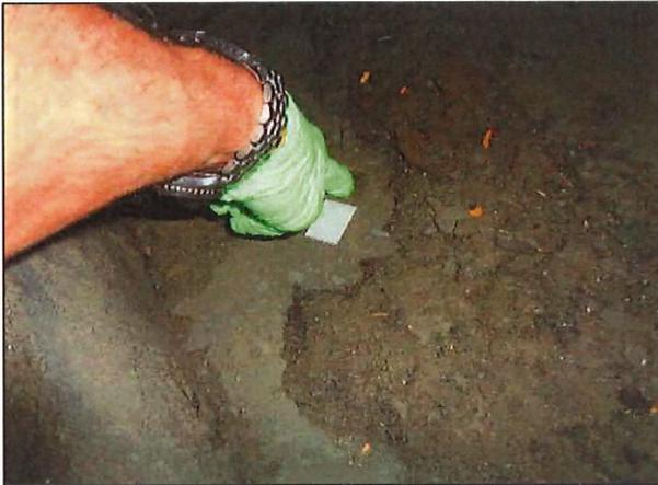
**Figure (7)** – Convention Center HVAC Unit #49 Tape Lift Sample #CC-2 in Return Air System.
