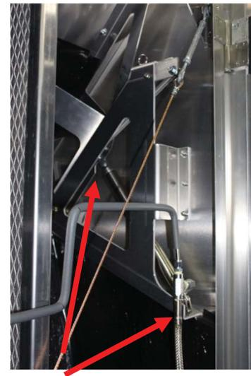
Figure 35. Louver Lubrication Points
