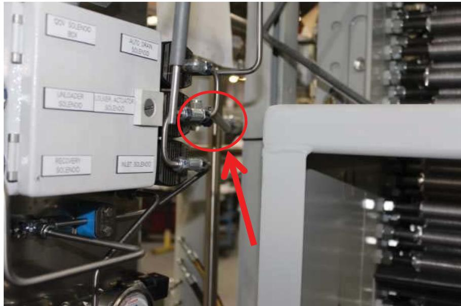
*Figure 12. Flow Control Valve*
