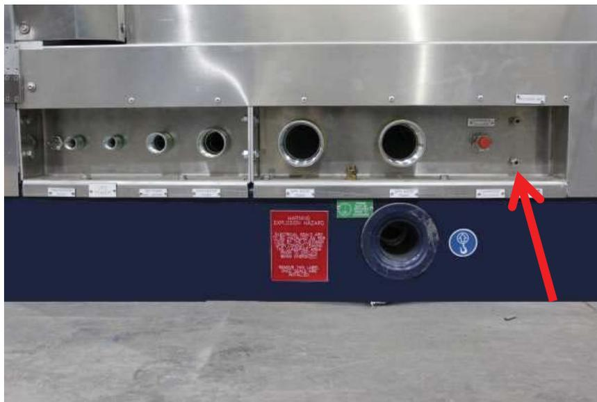
**Figure 13.** Connection Panel – Pilot Pressure In
