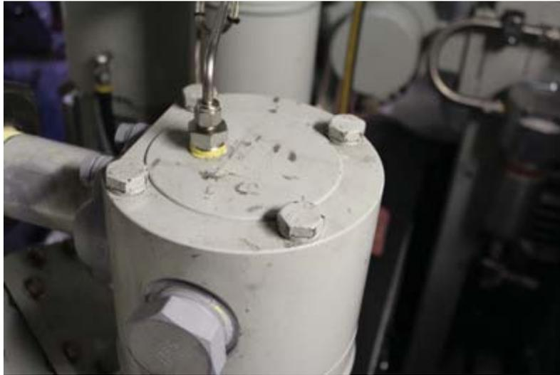
*Figure 26. Inlet Filter: Remove screws to access filter element*
