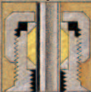
C. Adjustable Teflon ® stem packing
