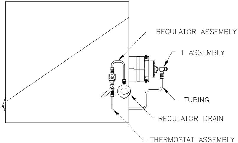
**Figure 2-44 Regulator Assembly Installed**
