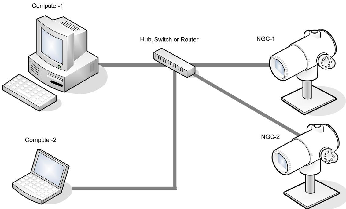
**Figure 3–1 Ethernet Connections**
