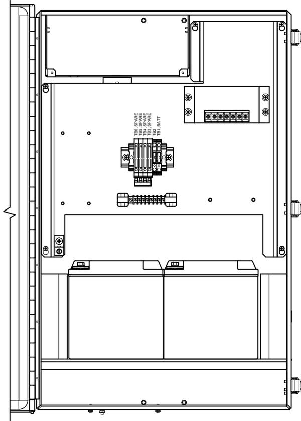
**Figure 2–63 Optional 6800 Enclosure with Battery Pack**
