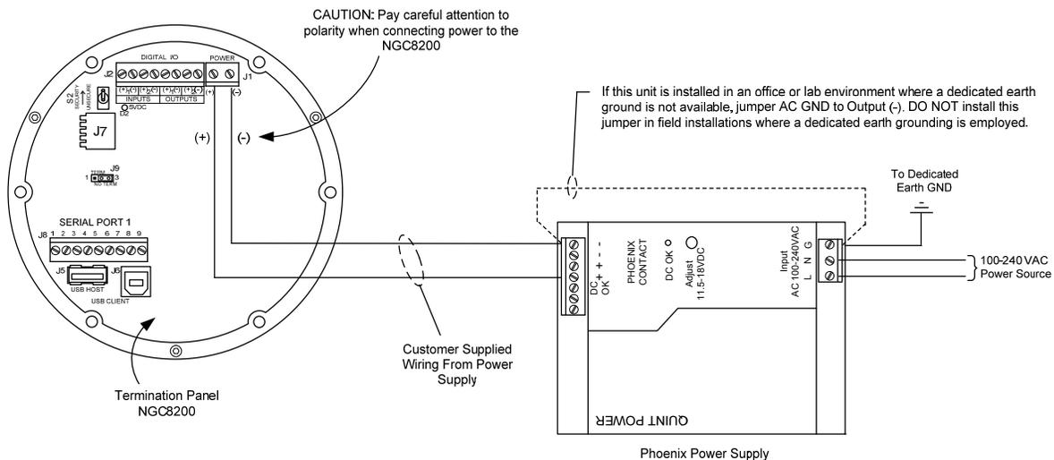
**Figure 2–61 AC/DC Converter Wiring Instructions**
