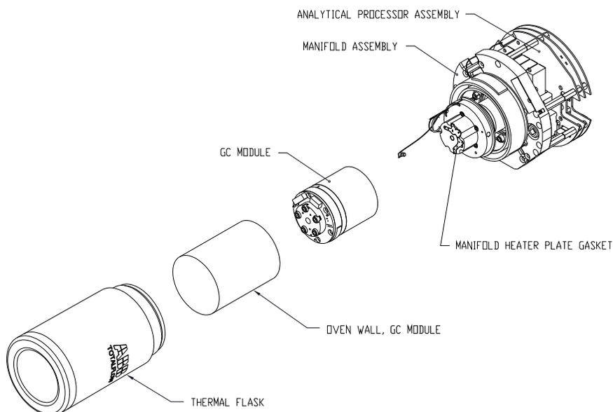
**Figure 4–8 GC Module, Exploded View**
