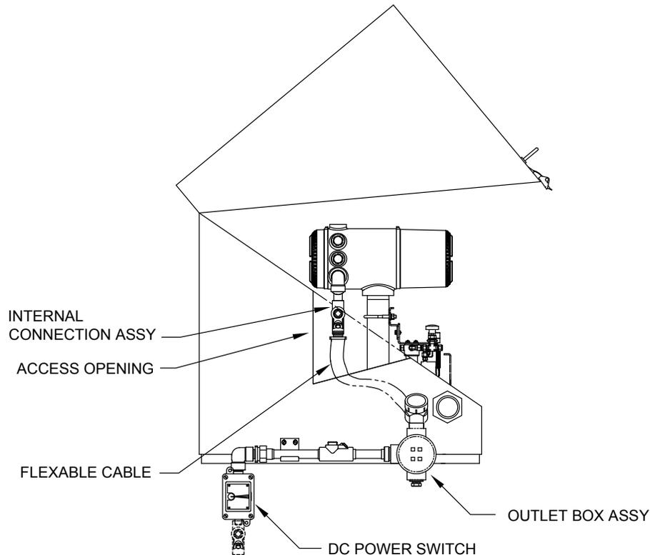
**Figure 2–24 CWE Access Panel Removed**
