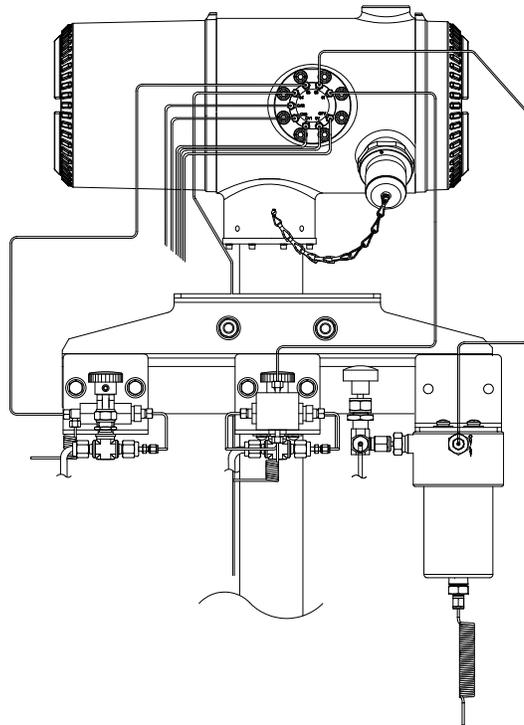
**Figure 1–23 Multiple Stream Sample Conditioning Assembly**
