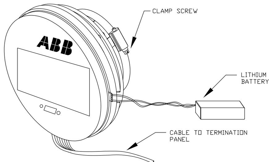
**Figure 4–4 Digital Controller Complete Assembly**
