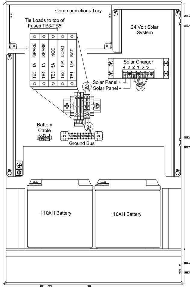
**Figure 1–28 6800 Enclosure with 24 VDC Solar Panel Power Supply Option**
