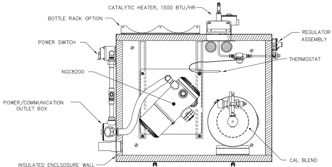
**Figure 1-20 NGC8200 Cold Weather Enclosure Installation w/ Catalytic Heater**
