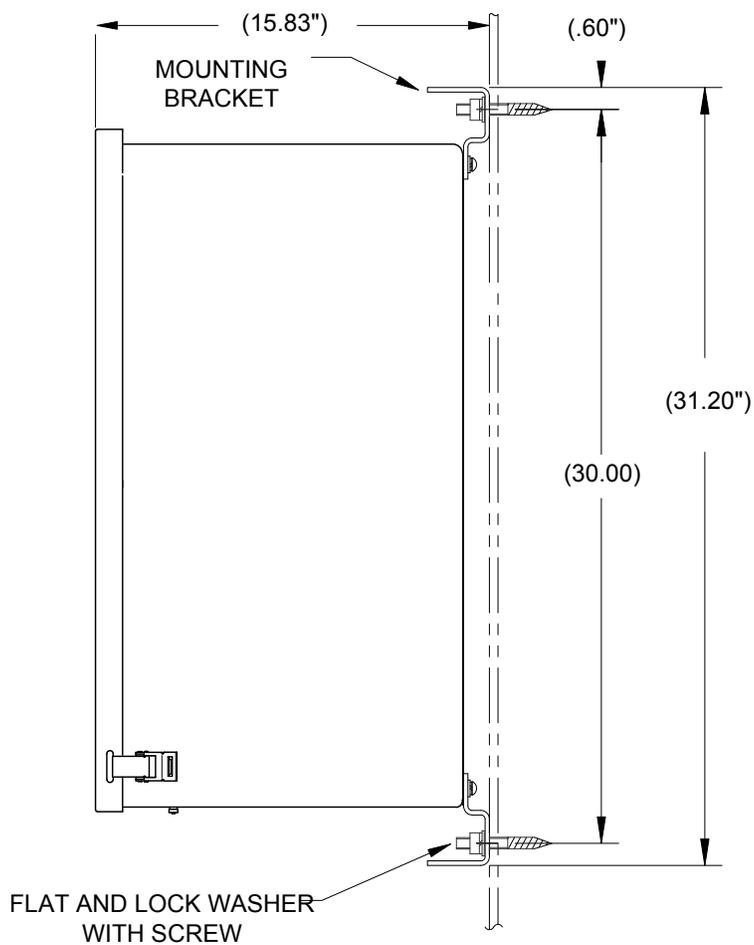
**Figure 2-54 6800 Enclosure Wall Mounted Installation**
