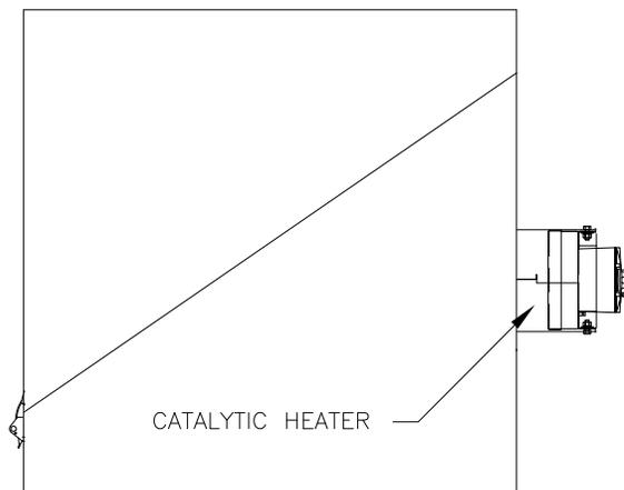
**Figure 2–41 Catalytic Heater Option in Cold Weather Enclosure**
