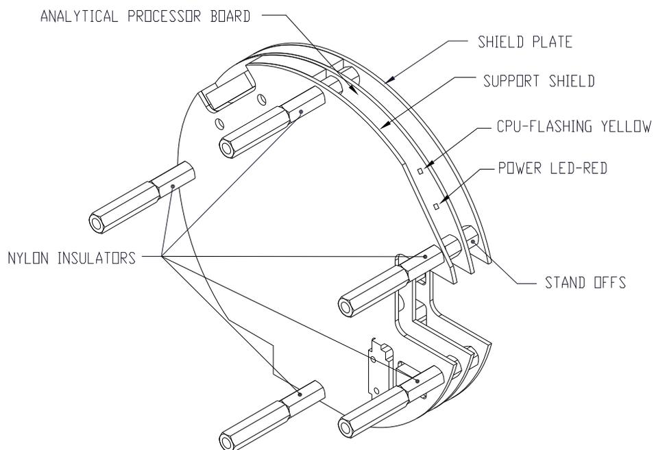
**Figure 1–11 Analytical Processor Assembly**
