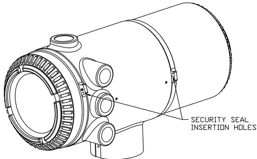
**Figure 1–26 NGC End Cap Tabs for Security Seal**
