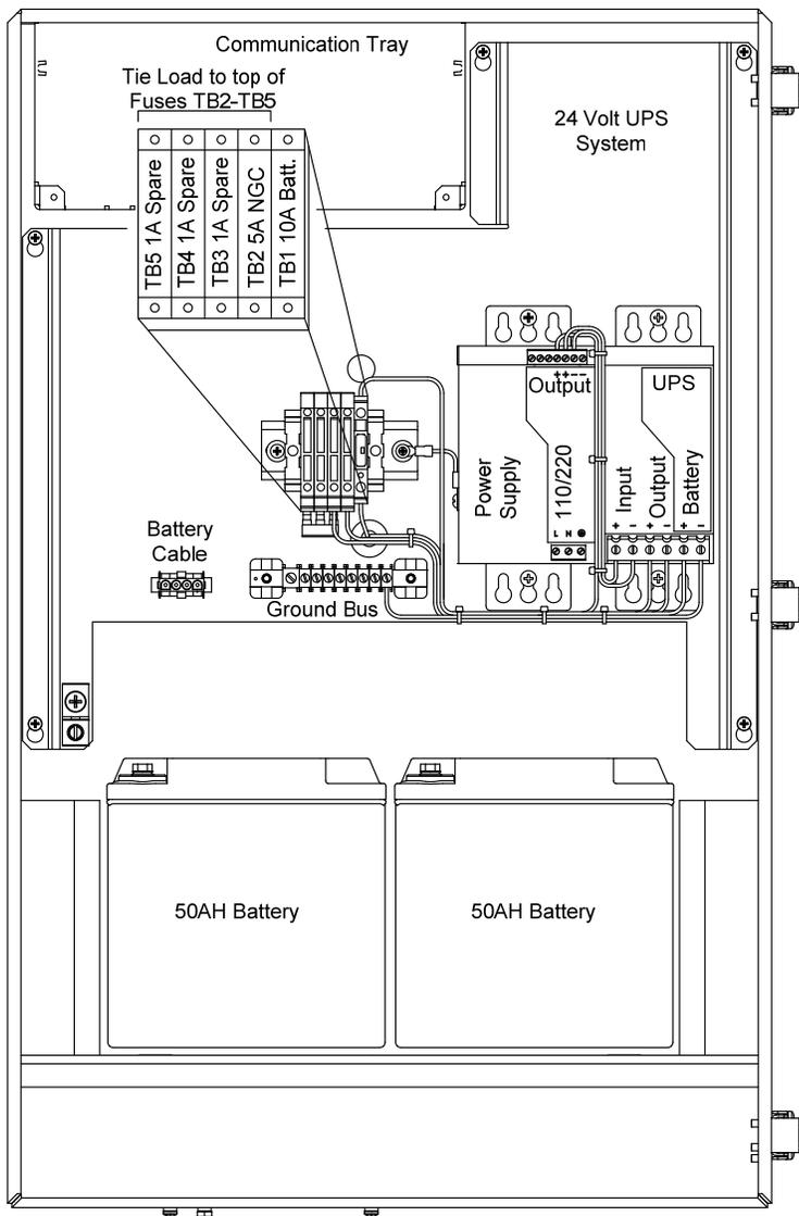
**Figure 1–29 6800 Enclosure with 115/230 VAC UPS Power Option**
