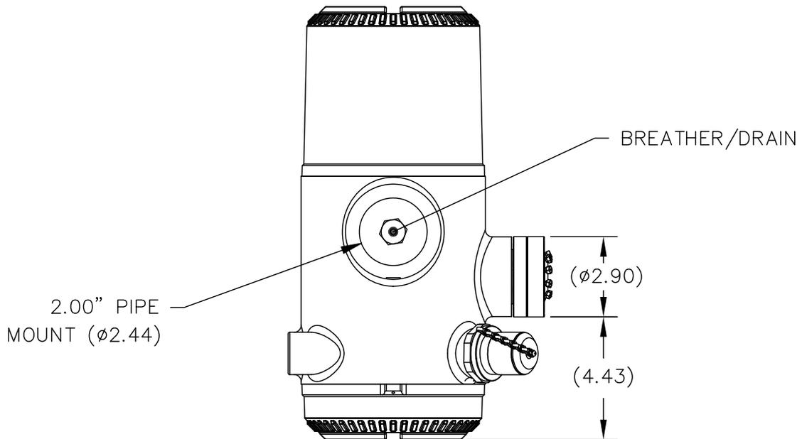
**Figure 1-7 NGC8206 Enclosure Underside**
