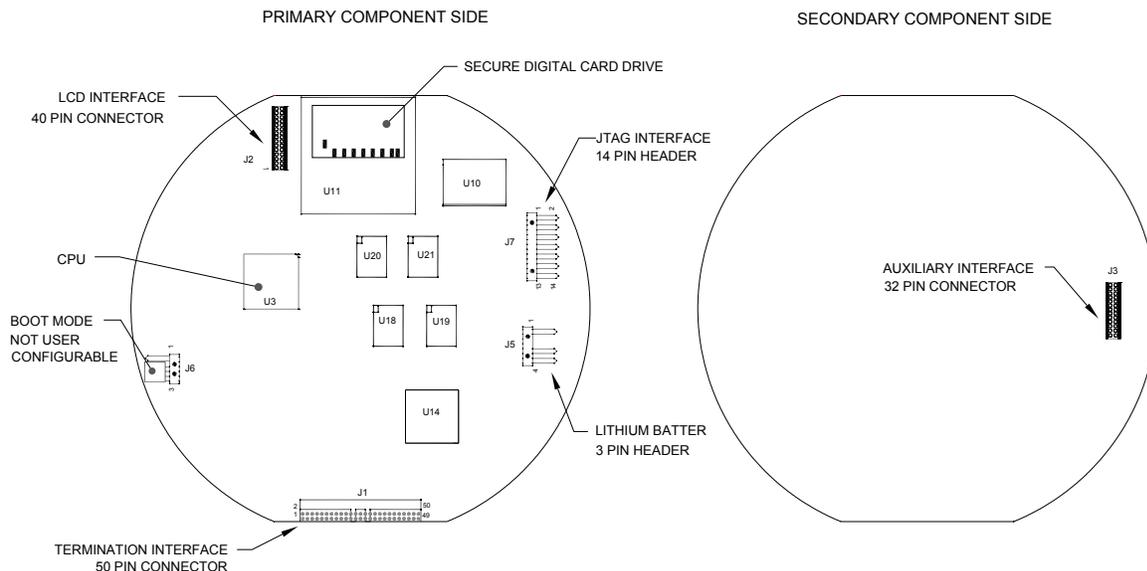
**Figure 4–5 Digital Controller Board**
