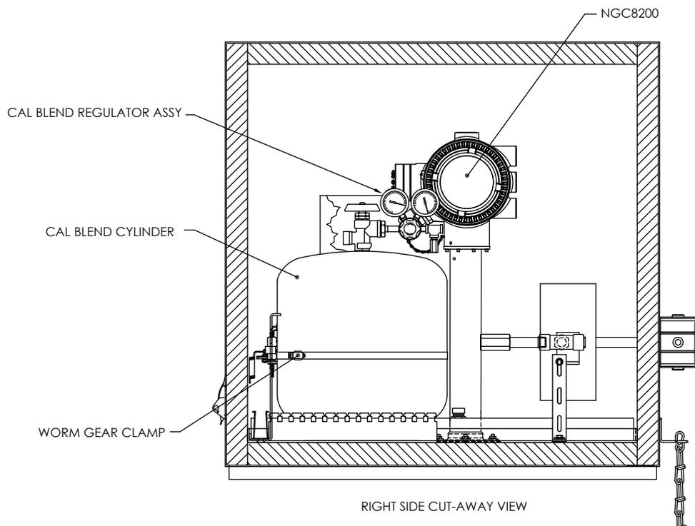
**Figure 2–36 Calibration Bottle Location**
