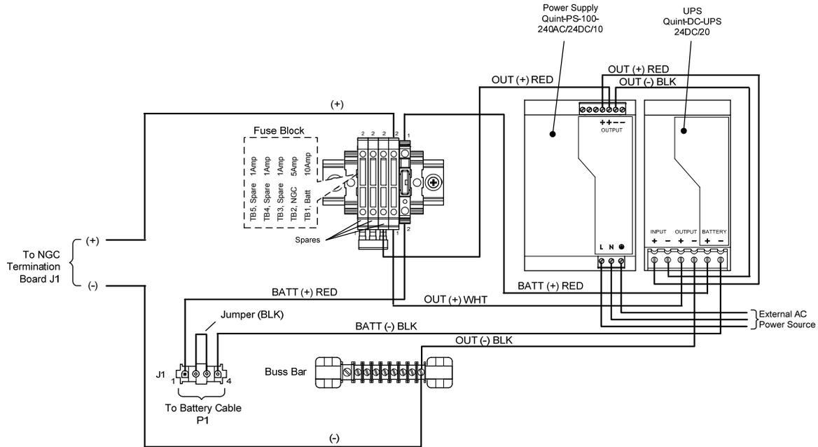
**Figure 2–55 115/230 VAC UPS Power Supply Option**
