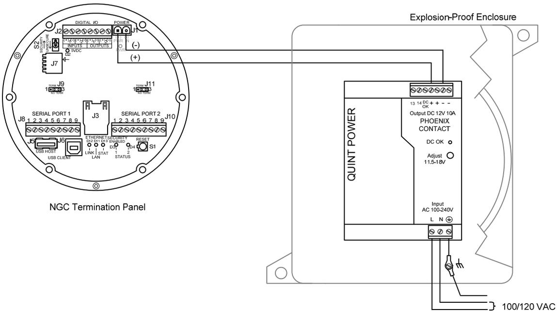
**Figure 2–58 Explosion Proof AC Power Supply Wiring Instructions**
