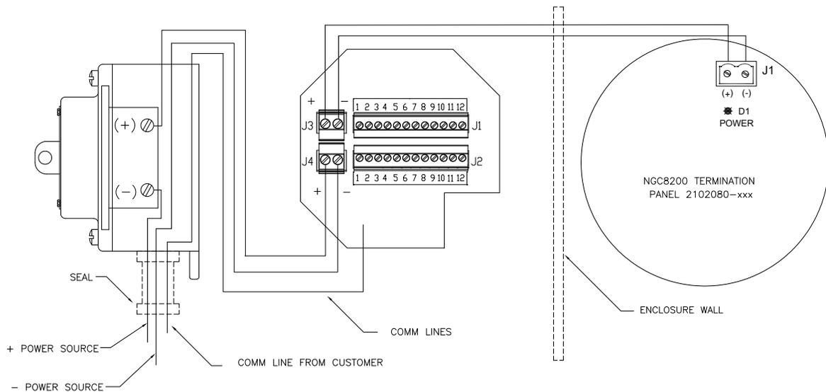
**Figure 2-27 Power Wiring Diagram**
