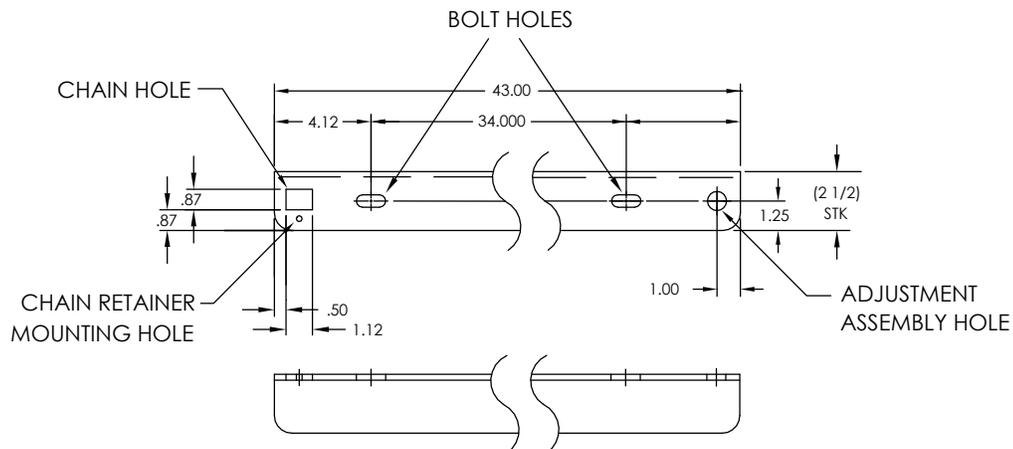
**Figure 2–8 Mounting Brackets**
