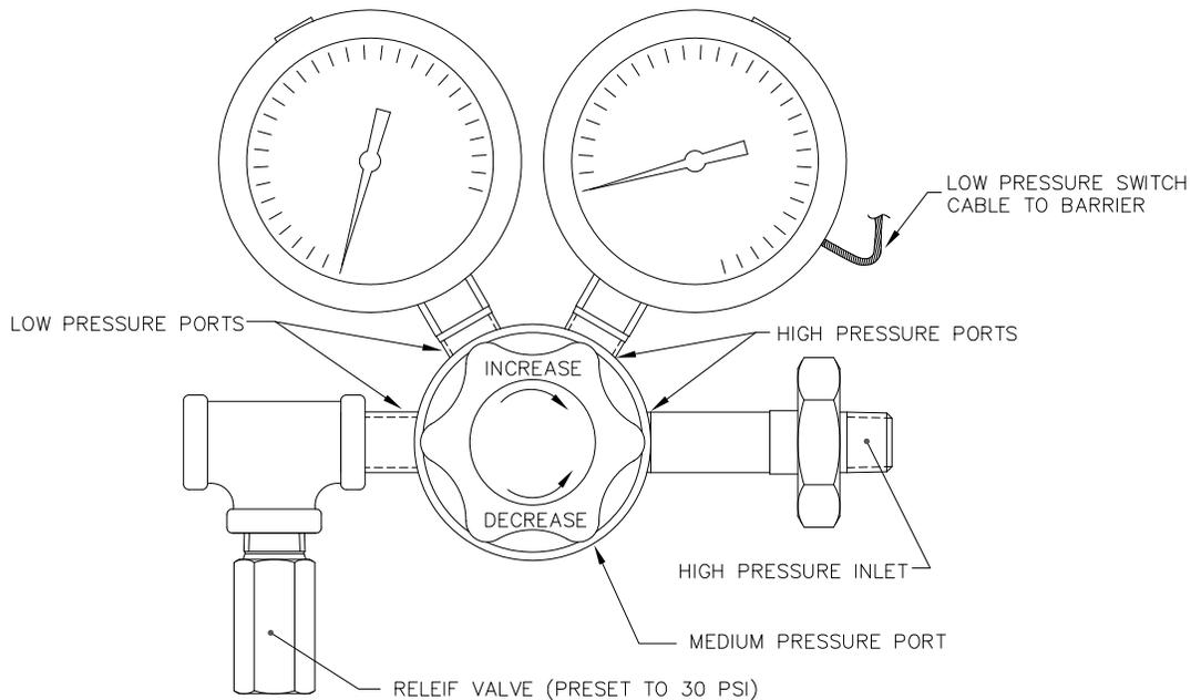
**Figure 2–37 Calibration Gas Pressure Regulator with Relief Valve**
