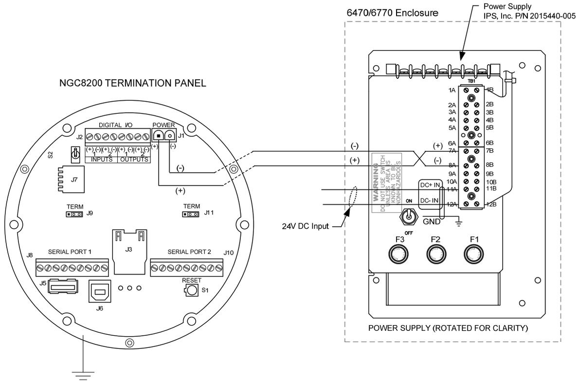
**Figure 2-62 24 VDC/12 VDC Power Supply Converter**
