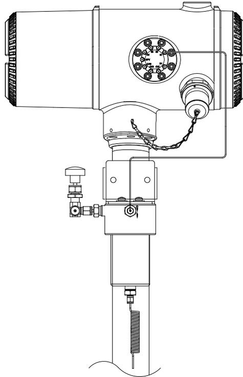
**Figure 1–22 Single Stream Sample Conditioning Assembly**
