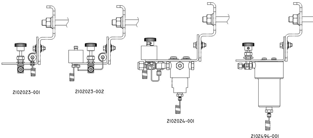
**Figure 2–20 Sample Conditioning Module Bracket**
