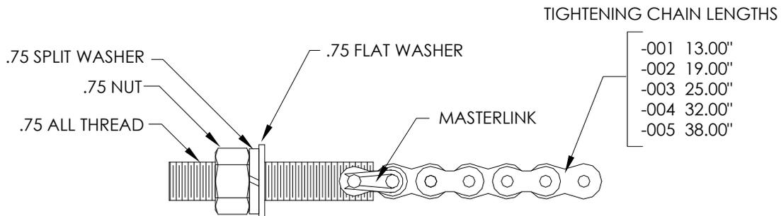
**Figure 2-10 Adjustment Assembly**
