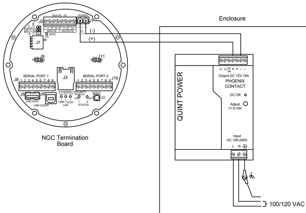
**Figure 5–4 AC Charger/Power Supply Wiring**
