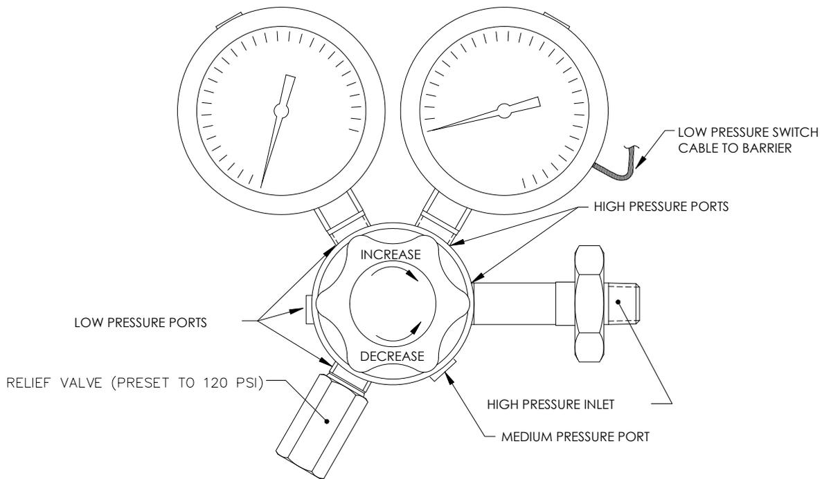
**Figure 2–34 Carrier Gas Pressure Regulator with Relief Valve**
