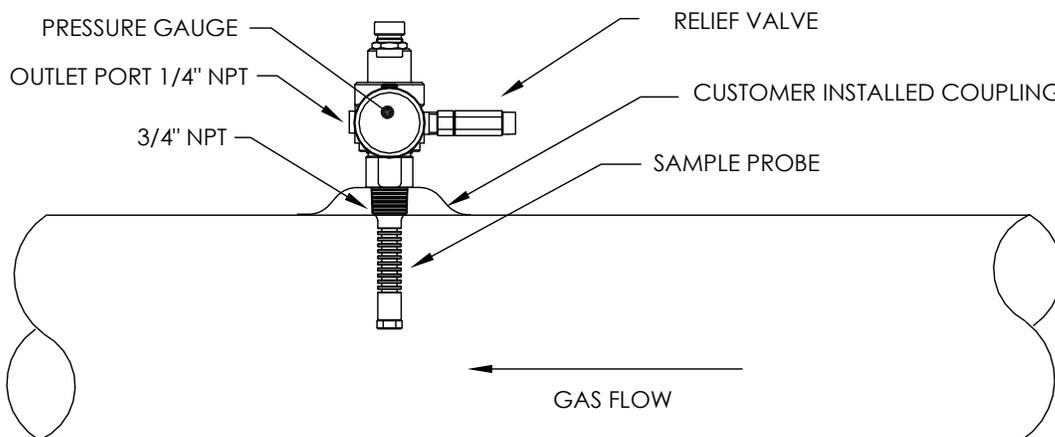
**Figure 1–18 Temperature Compensated Regulator With Sample Probe**
