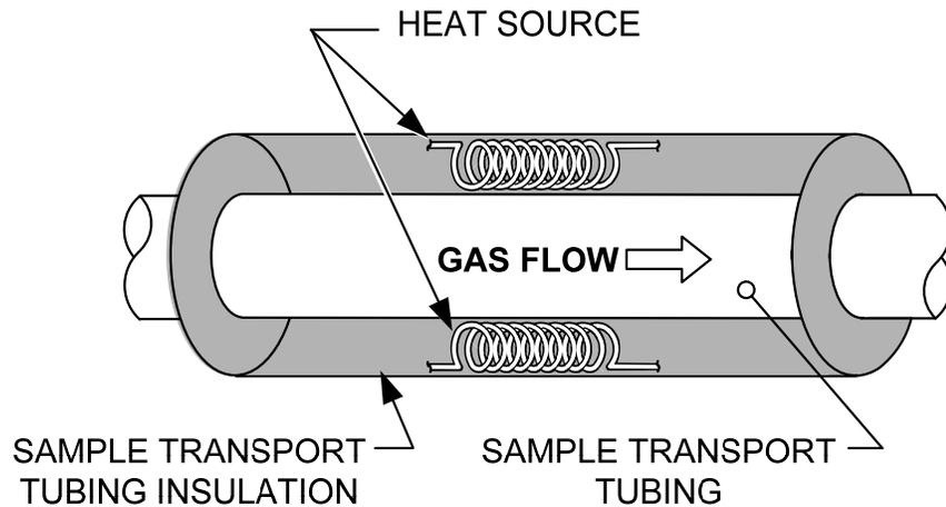
**Figure 1–16 Heat Tracing Sample Line**
