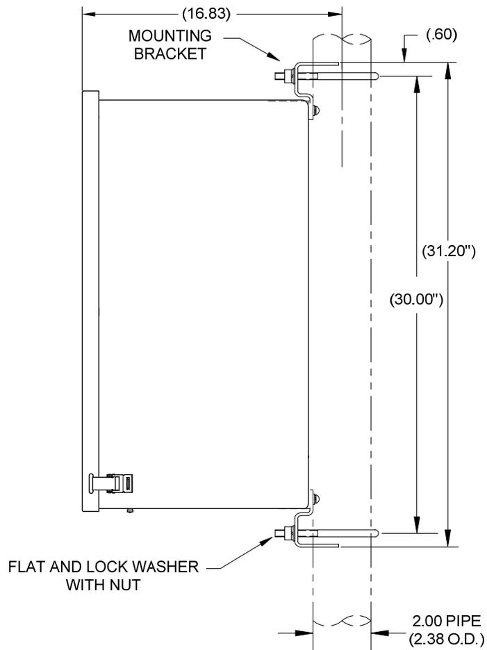
**Figure 2-51 6800 Enclosure Pipe Mounting Installation**
