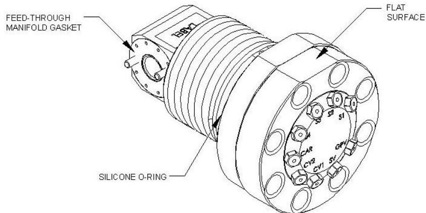
**Figure 4–10 Feed-Through Assembly**
