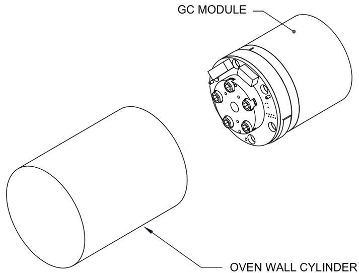
**Figure 1–12 GC Module Assembly**
