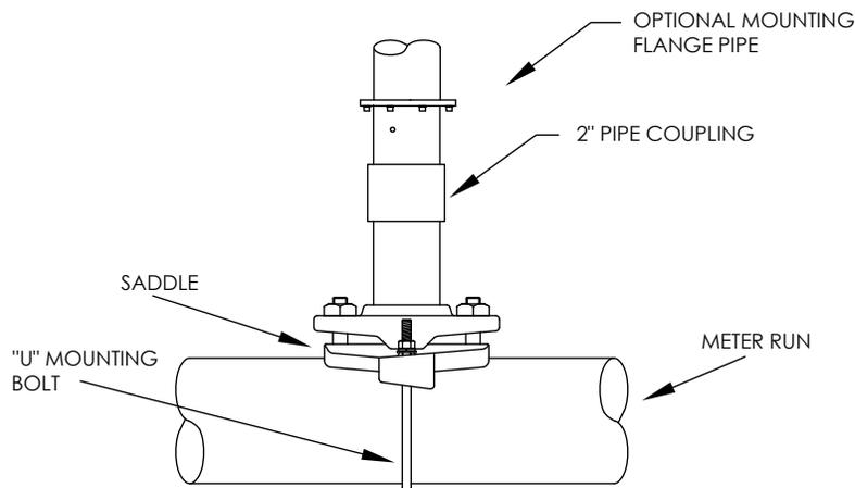
**Figure 2–14 Typical Pipe Saddle Installation**
