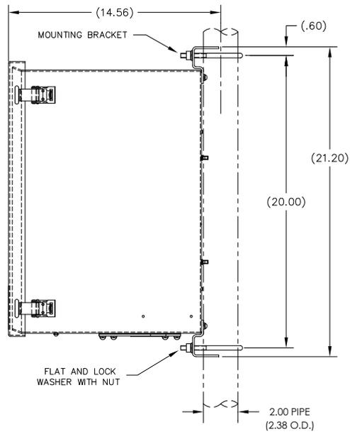
**Figure 2-50 6700 Enclosure Pipe Mounting Installation**
