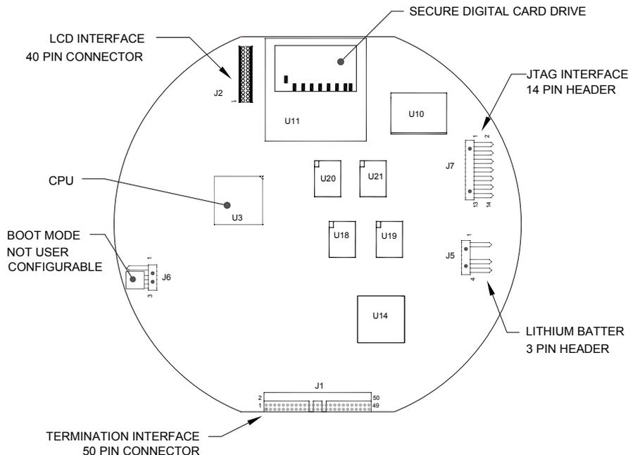
**Figure 4–11 Primary Component Side Digital Controller Board**
