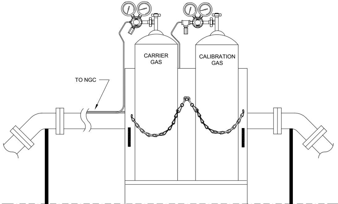
**Figure 2–31 Carrier/Calibration Gas Bottle Rack Installation**
