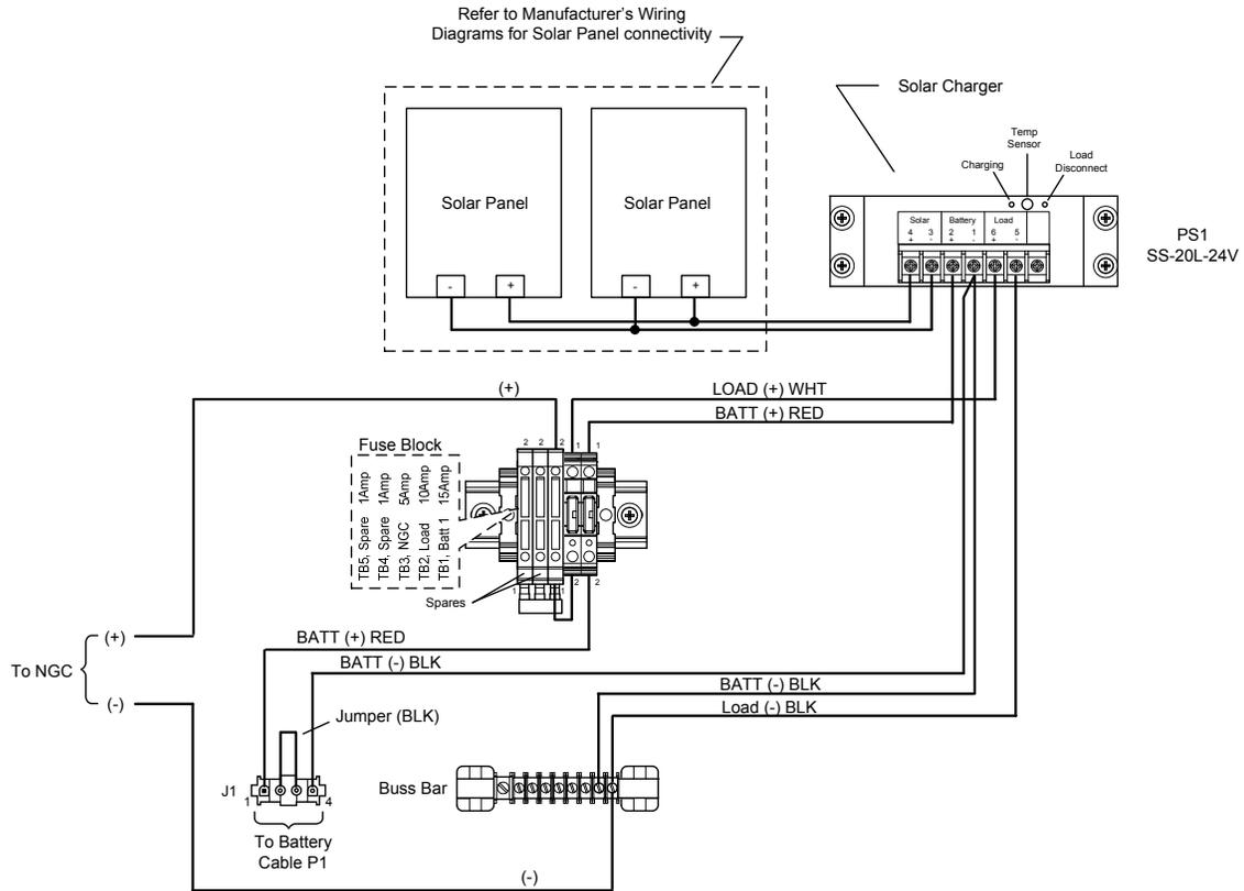
**Figure 2–67 24 VDC Solar Panel Power Supply**
