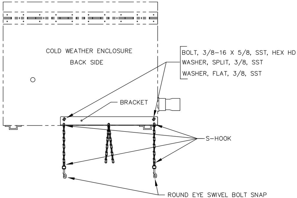
**Figure 2-33 Dual Bottle Rack Installation**
