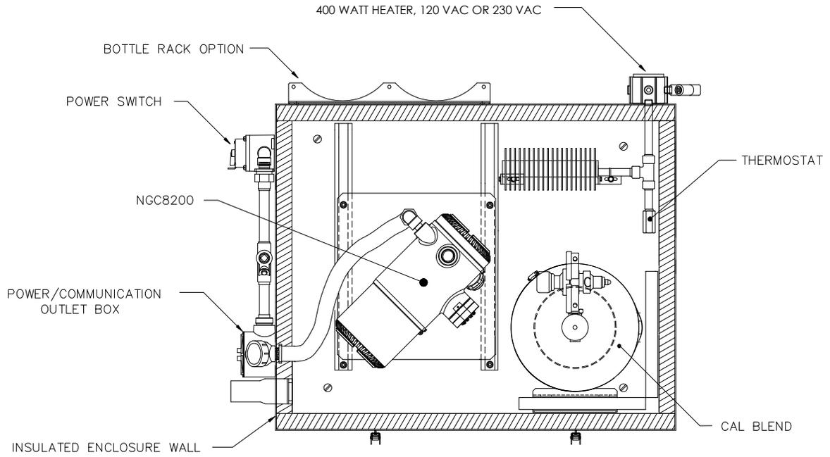
**Figure 2-47 Electrical Heater Installed in CWE**
