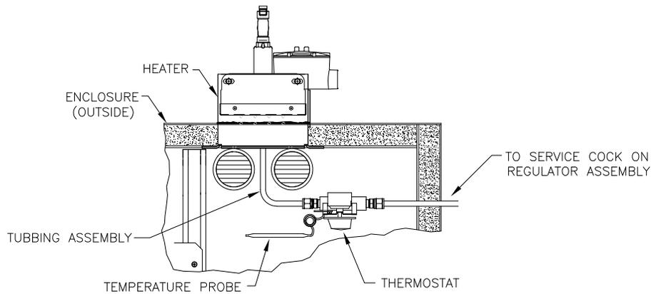
**Figure 2-43 Thermostat Assembly Installed**
