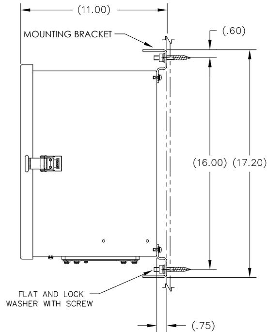
**Figure 2–52 6200 Enclosure Wall Mounted Installation**
