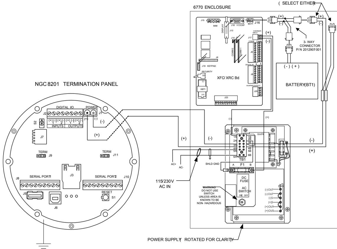
**Figure 2-65 Battery Pack with AC Power Supply Wiring Instructions**
