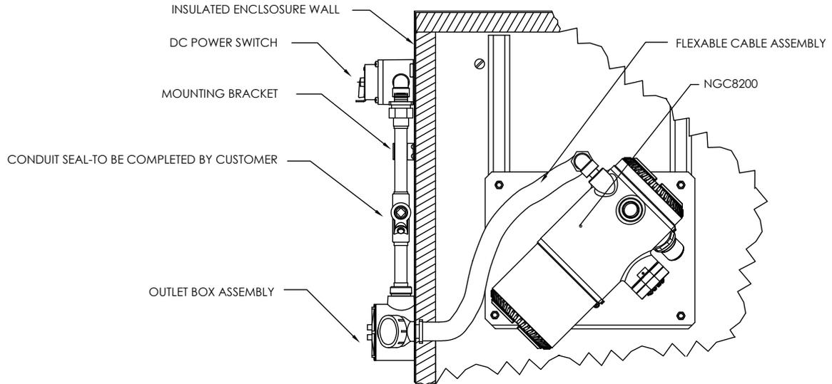
**Figure 2-26 Assembled Power/Communication Assembly**
