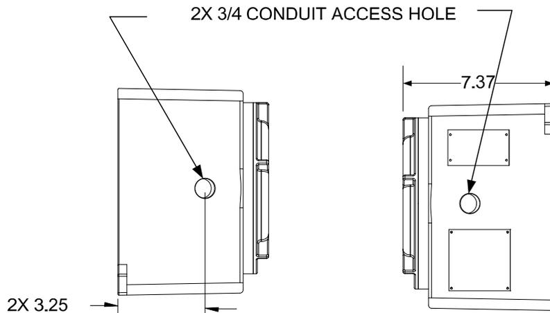
**Figure 2-57 Explosion Proof AC Power Supply Side Dimensions**
