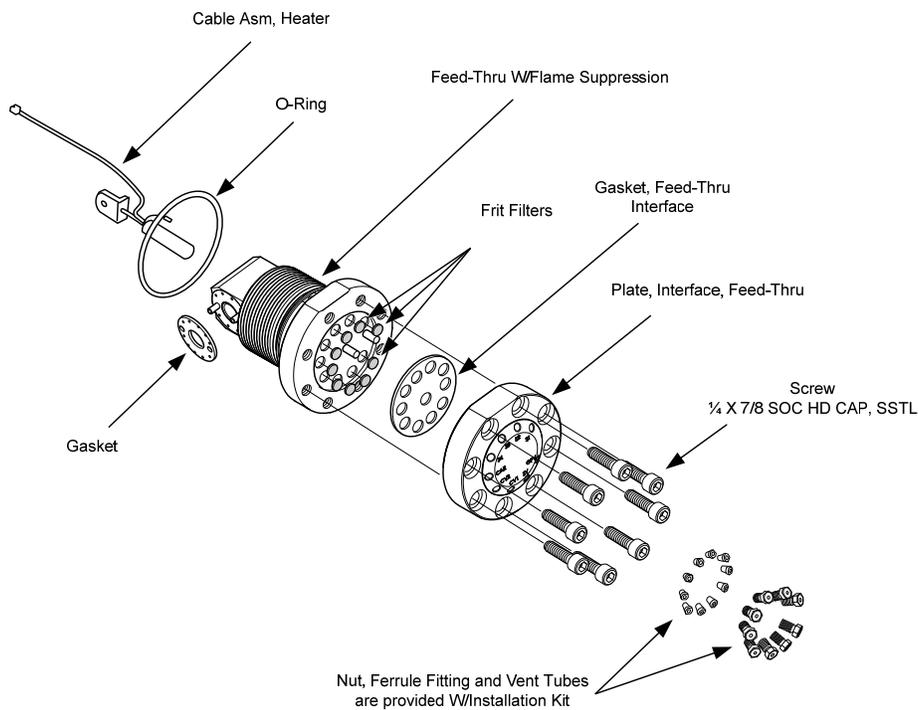
**Figure 4-3 Feed Through Assembly, Exploded**
