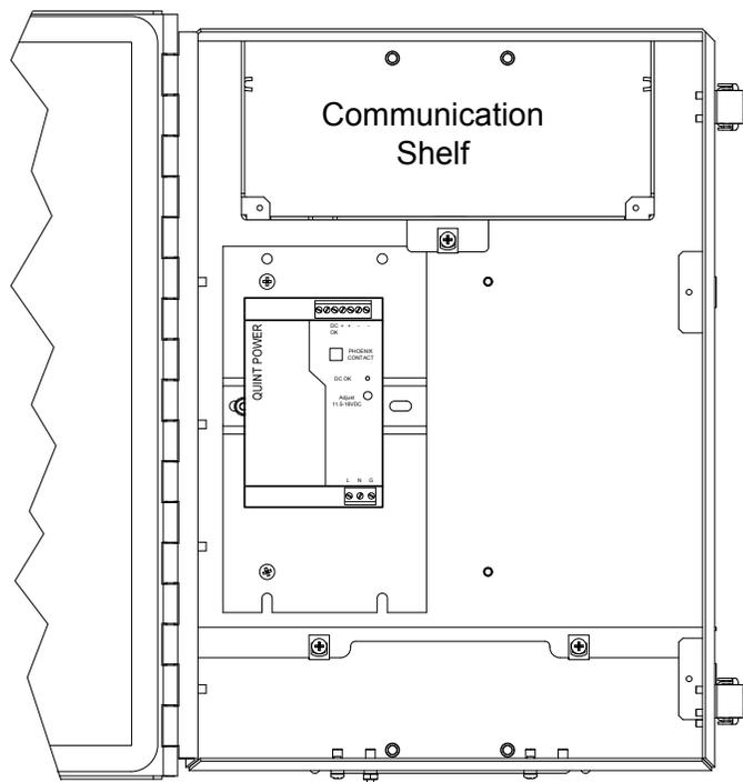
**Figure 2-60 6700 Optional Equipment Enclosure with Power Supply**
