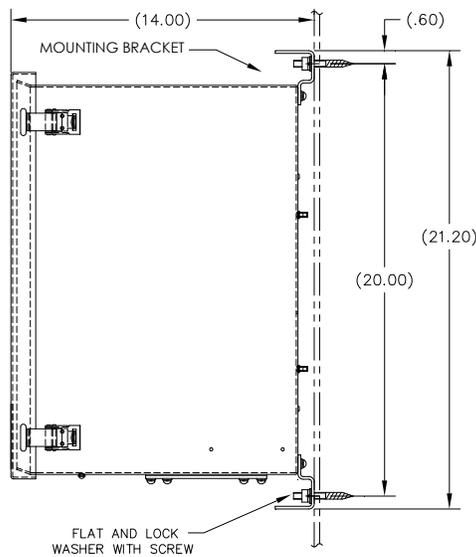
**Figure 2-53 6700 Enclosure Wall Mounted Installation**
