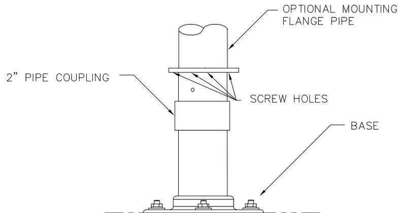
**Figure 2–19 NGC Optional Mounting Flange Pipe**
