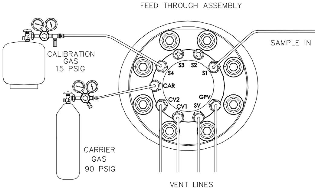
**Figure 2–40 Vent Line Connections on Feed-through Assembly**
