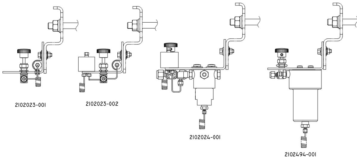
**Figure 1–21 Available Sample Conditioning Modules**
