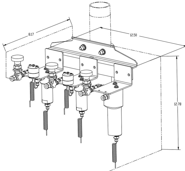
**Figure 1–25 Multiple Stream Conditioning Module Dimensions**
