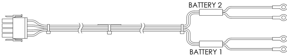
**Figure 2–64 24 VDC Dual Battery Pack Cable**
