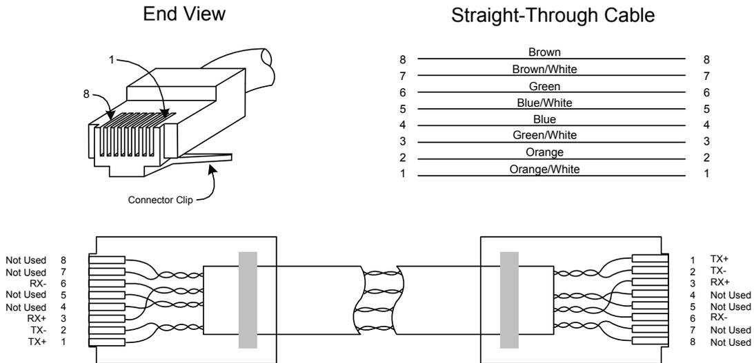
**Figure 3–2 Ethernet Cable-Typical**
