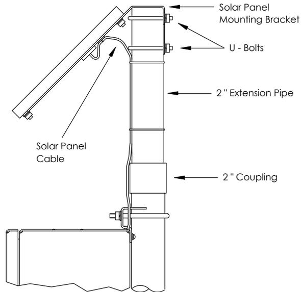
**Figure 2–66 Typical Solar Panel Installation**
