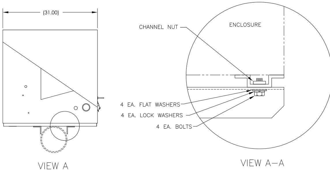
**Figure 2-9 Mounting Hardware Installation**
