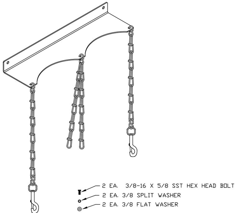
**Figure 2-32 Dual Bottle Rack Assembly**
