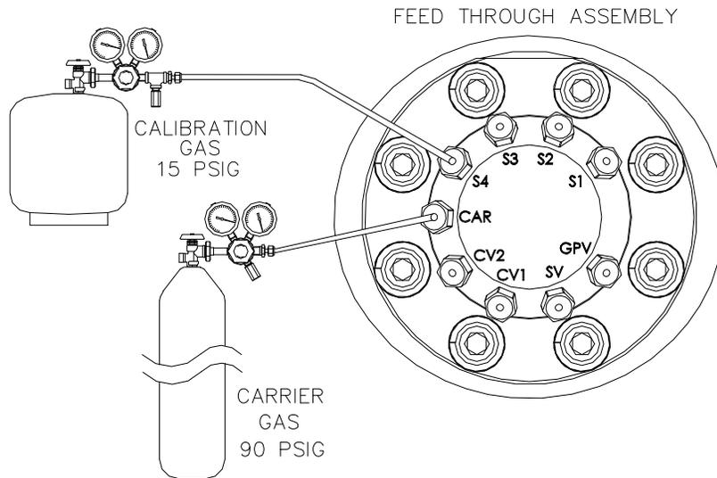
**Figure 2–39 Carrier and Calibration Gas Connections**
