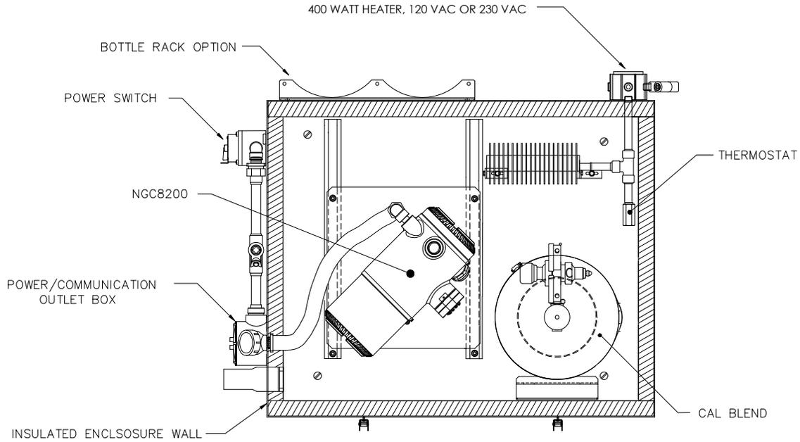
**Figure 2–3 Typical Cold Weather Enclosure with Electrical Heater**
