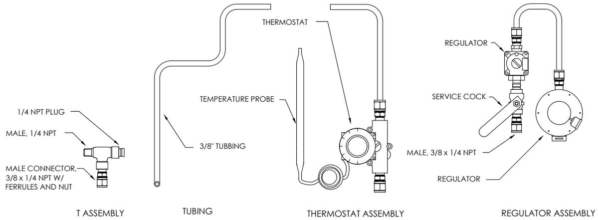
**Figure 2-42 Catalytic Heater Assembly**
