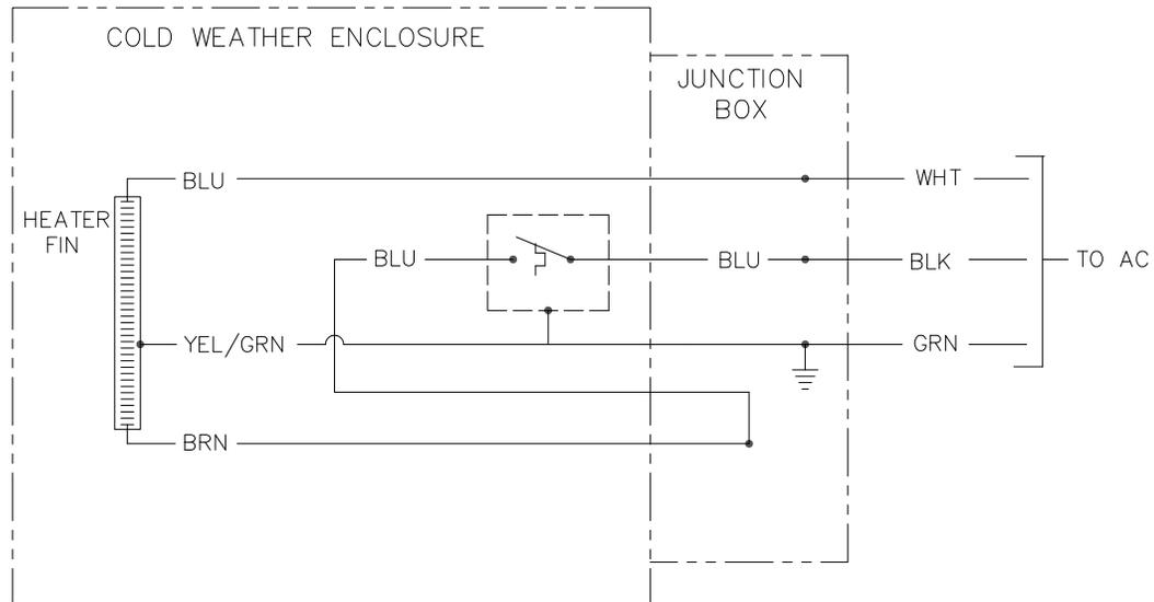
**Figure 2-48 Electric Heater Option Wiring Instructions**
