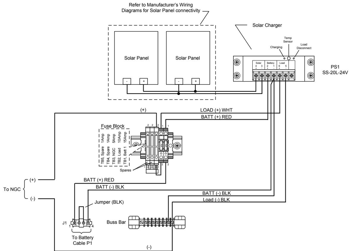
**Figure 5–3 Solar Panel Wiring Instructions**
