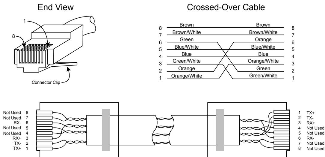
**Figure 3–3 Ethernet Cable-Cross-Over**
