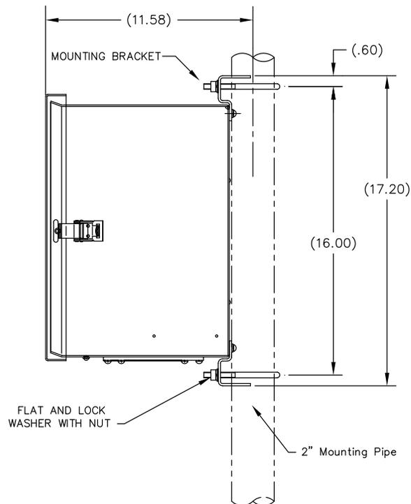
**Figure 2-49 6200 Enclosure Pipe Mounting Installation**
