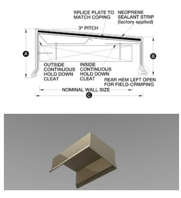
The coping cap shall have fabricated end caps as illustrated and made part of the warranted assembly.
