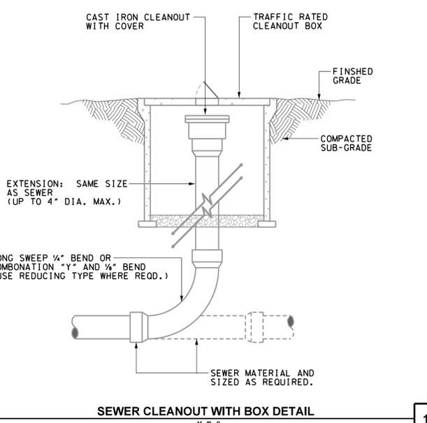
SEWER CLEANOUT WITH BOX DETAIL
