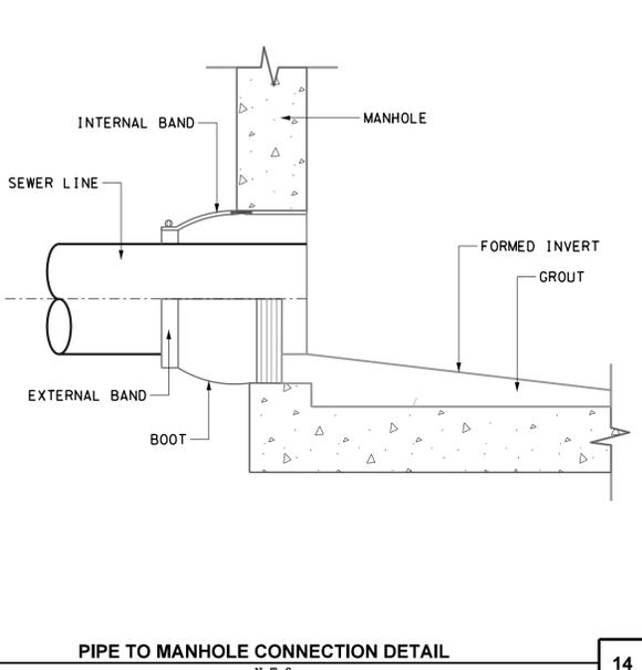
PIPE TO MANHOLE CONNECTION DETAIL
