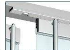
Rail Mount Detail at Latch with Header and EBK Strike
