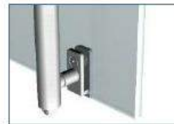
Glass Mount Detail at Latch
