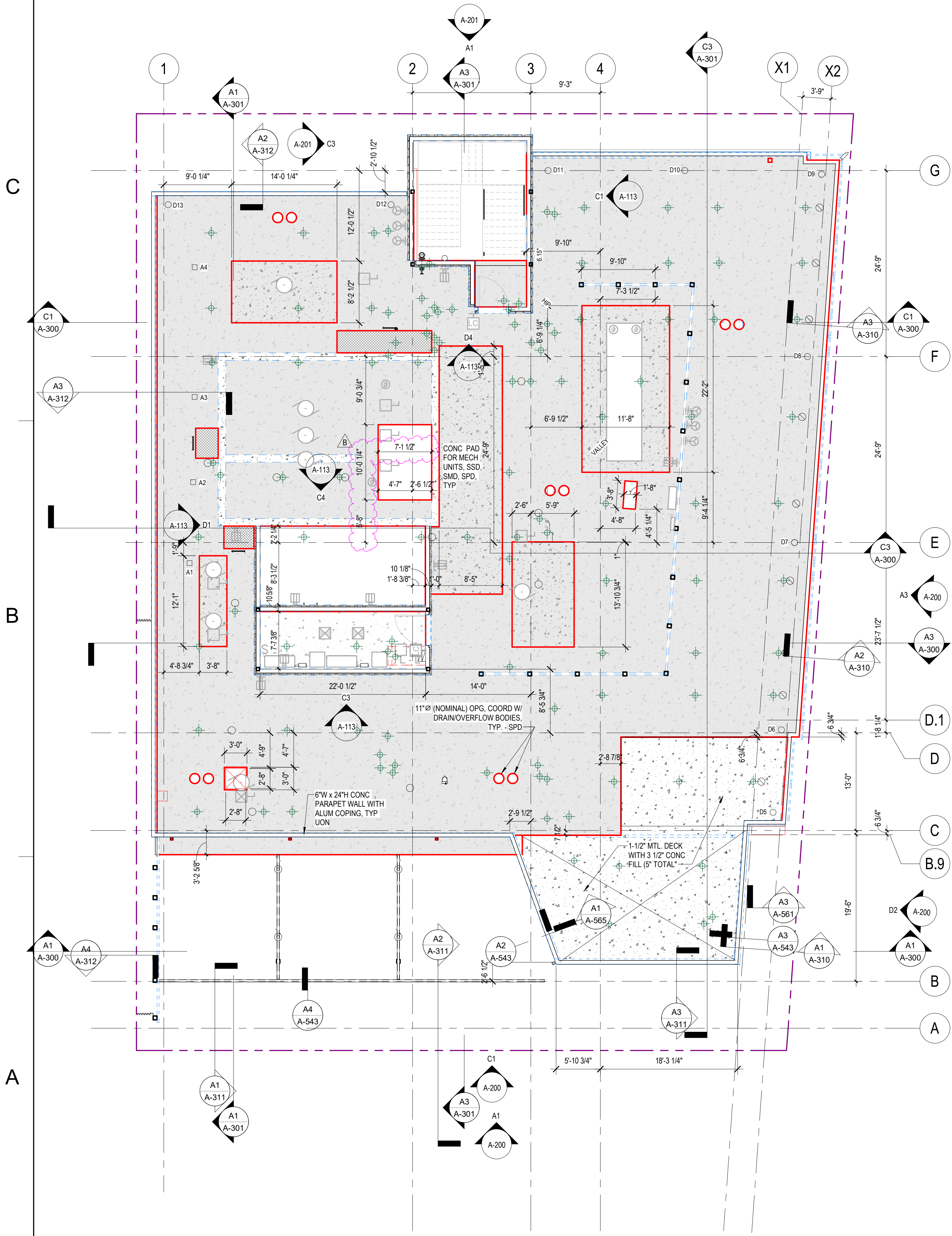
A1 ROOF - EDGE OF SLAB PLAN 1/8" = 1'-0"
