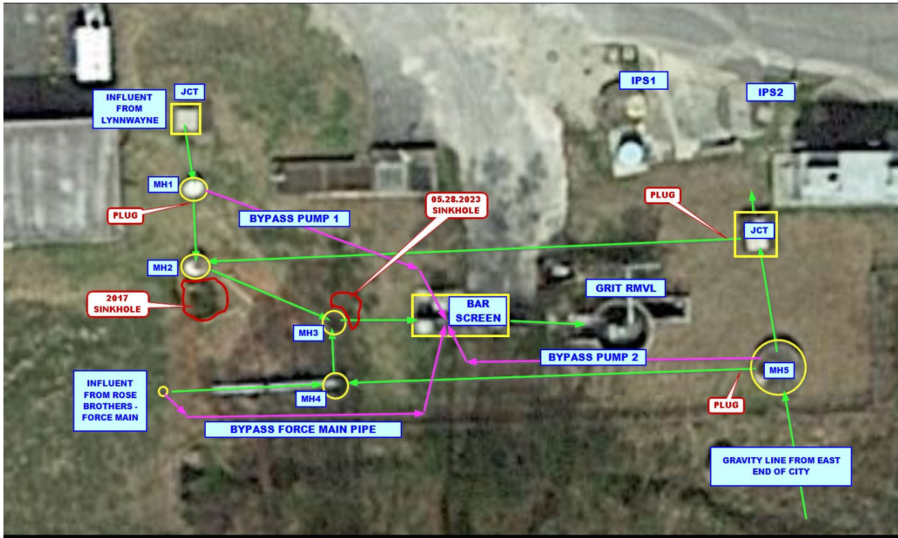
Figure 2: Bypass diagram and sewer flow diagram
