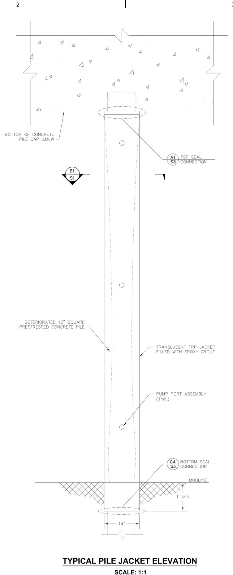
**TYPICAL PILE JACKET ELEVATION**
