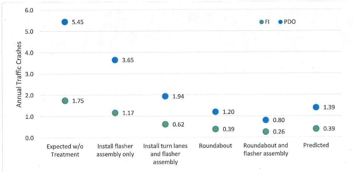
**Figure 12. Safety Impact of Various Treatment Scenarios – SR-53 at New Cut/Ednaville Road Intersection**
