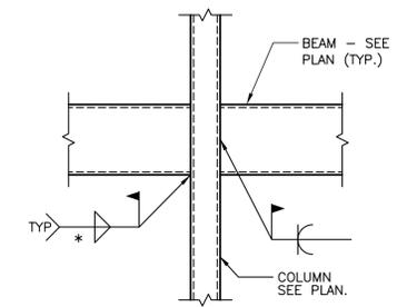
**TYPICAL TUBE BEAM TO COLUMN CONNECTION (BEAM TO FACE OF COLUMN)** 8
