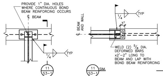
**TYP. BEAM BEARING ON CMU WALL IN PLAN VIEW** 10
