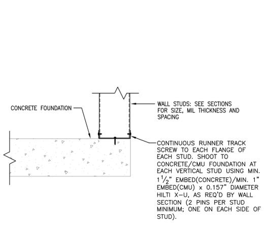
SECTION DETAIL: TRACK TO SLAB
