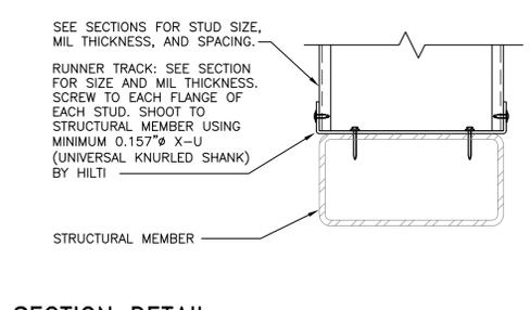
SECTION DETAIL: TRACK TO STRUCTURAL STEEL
