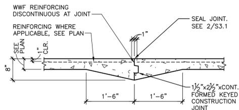
**TYPICAL CONSTRUCTION JOINT SLABS ON GRADE** 3
