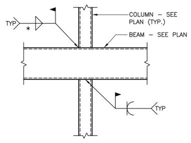
**TYPICAL TUBE BEAM TO COLUMN CONNECTION (BEAM TO FACE OF COLUMN)** 9
