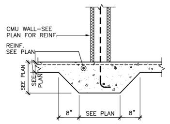
**TYP. THICKENED SLAB AT INTERIOR WALLS** 6
