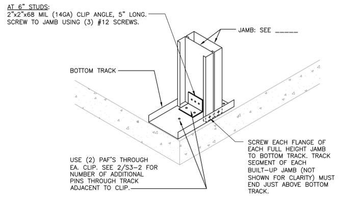
JAMB TO SLAB AT OPENINGS
