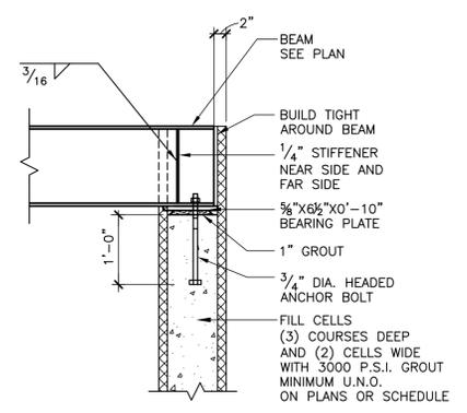
**TYPICAL BEAM BEARING PERPENDICULAR ON CMU WALL** 11
