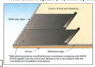
System # 1- Apply a Self-Adhering Polymer-Modified Bitumen underlayment complying with ASTM D1970 applied over entire roof deck.
