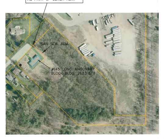
SEWER, REM LESS THAN 24" 115 FT TREE, REM. 6"-18" 1 EA. SIDEWALK, REM. BUILDING DEMO. WELL ABANDONMENT TURF RESTORATION
