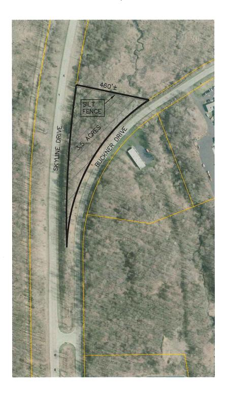
CLEARING & GRUBBING 3.5 ACRE EROSION CONTROL, SILT FENCE 550 FT TURF RESTORATION 16,940 SYD
