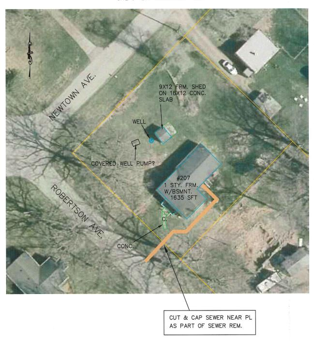
SEWER, REM LESS THAN 24" 75 FT SIDEWALK, REM. BUILDING DEMO. WELL ABANDONMENT TURF RESTORATION
