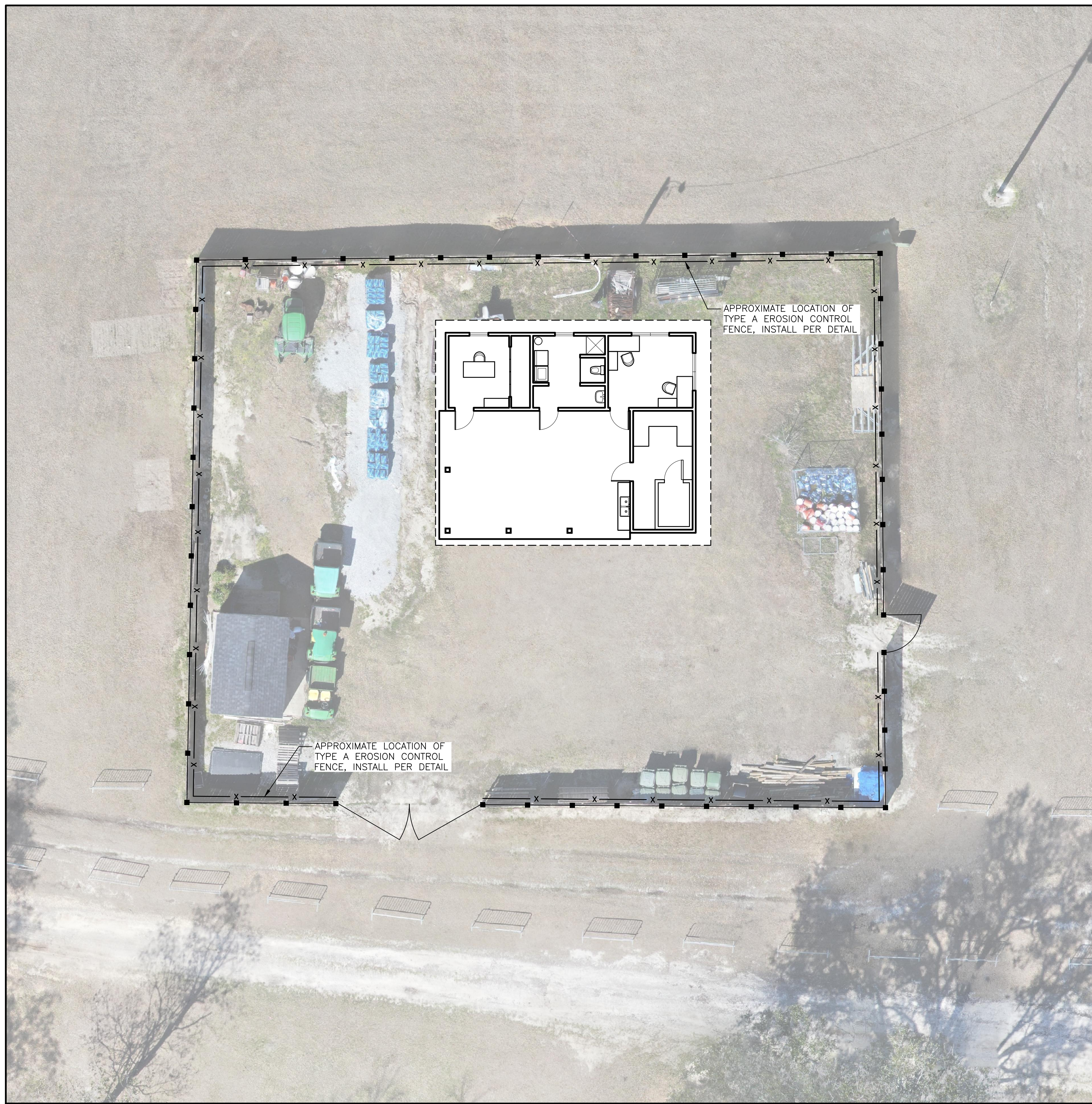
1 EROSION AND SEDIMENTATION CONTROL PLAN Scale: 1" = 10'
