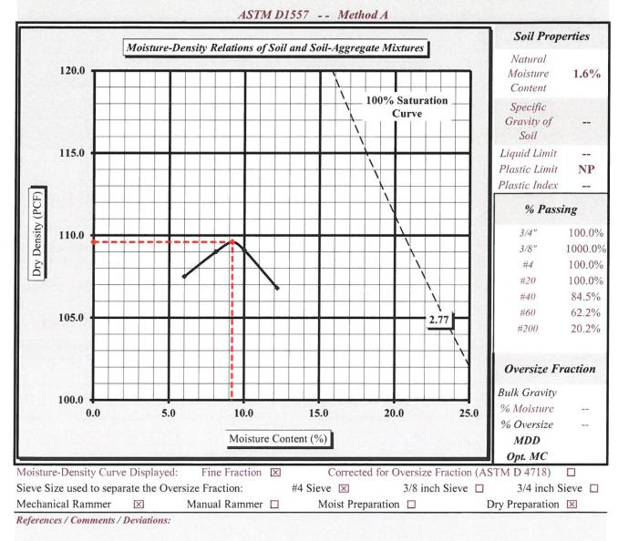
ASTM D 2216: Laboratory Determination of Water (Moisture) Content of Soil and Rock by Mass ASTM D 1557: Laboratory Compaction Characteristics of Soil Using Modified Effort
