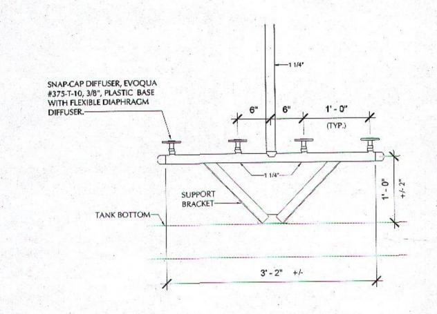
DIFFUSER HEADER ASSEMBLY DETAIL
