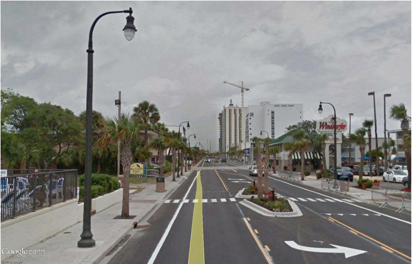
Example Photo, with Heritage Teardrop Luminaire on Davit (Streetlight Type Group L-2)
