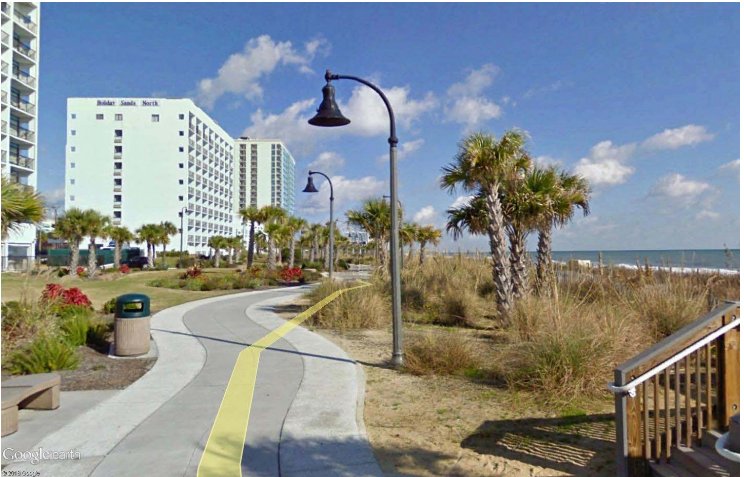
Example Photo, with Heritage Teardrop (Sag Glass, Deep Skirt) Luminaire on Davit (Streetlight Type Group L-3)
