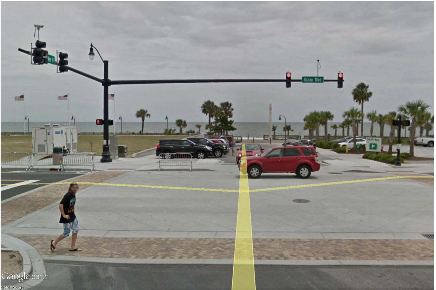
Example Photo; Type Group T-1p Pedestrian Pole also shown on right (Beach Pylon and Type Group L-3 Streetlights also appear in background)
