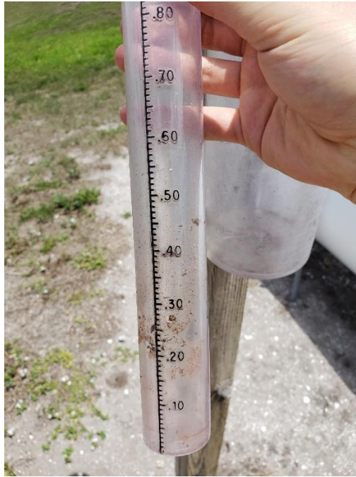
Figure 1-29 Rain Data Gauge Graduated Cylinder Inside the Canister
