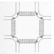
(Figure 8-9 FHWA). GOOD DESIGN: Continental markings should be used at all pedestrian crossings because research has determined that they are most visible to motorists.
