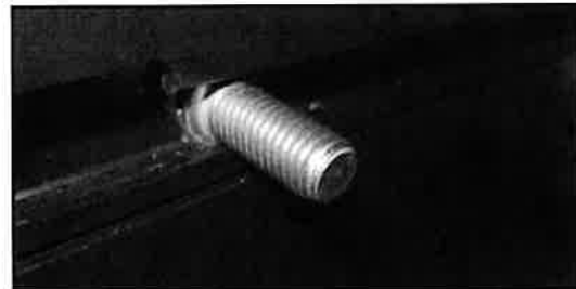
Figure 1 • Slim cabinet mounting bolt inserted in track.
