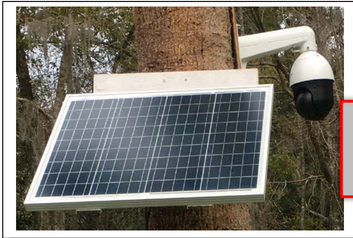
Camera unbolts from arm to prevent damage during mounting.
