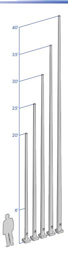
SHAFT: One-piece extruded 6063 aluminum alloy tube heat treated to a T6 temper. Shaft has a uniform taper.
