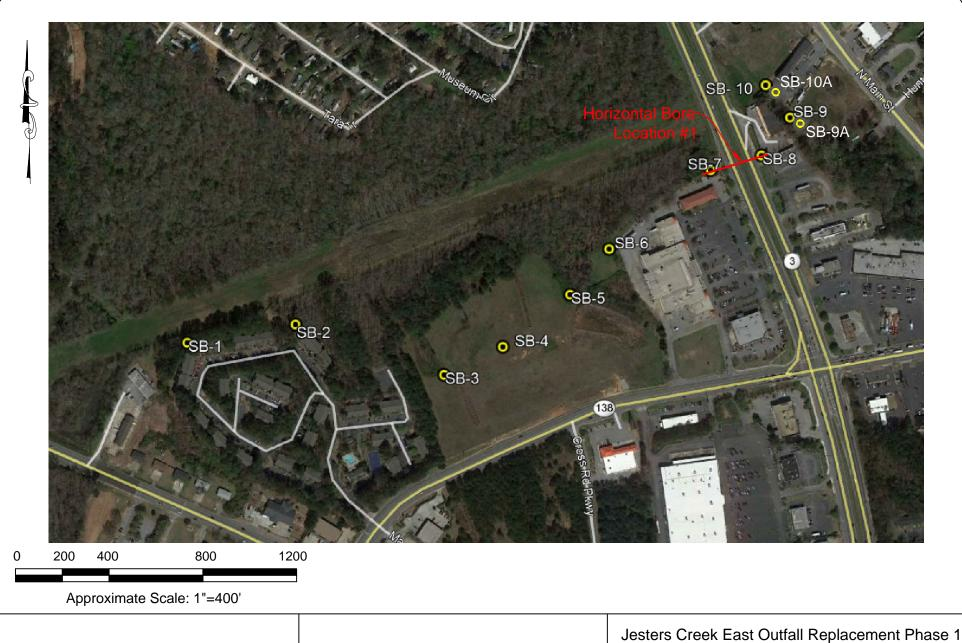
Figure 2: Boring Location Plan
