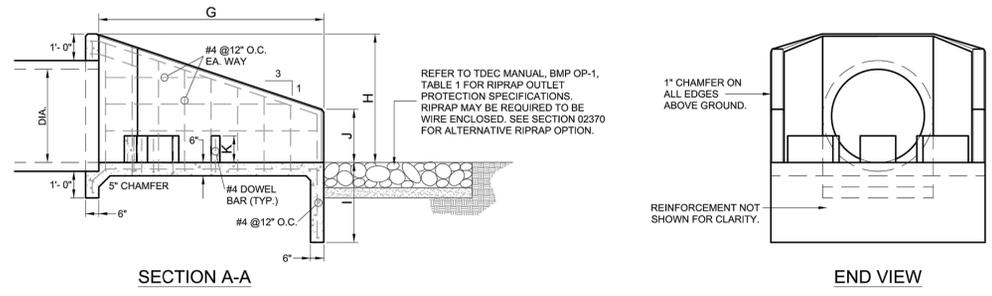
REFER TO TDEC MANUAL, BMP OP-1, TABLE 1 FOR RIPRAP OUTLET PROTECTION SPECIFICATIONS. RIPRAP MAY BE REQUIRED TO BE WIRE ENCLOSED. SEE SECTION 02370 FOR ALTERNATIVE RIPRAP OPTION.
