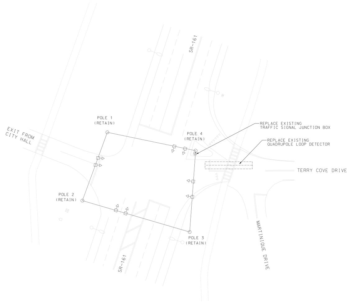
LOOP WIRE REMOVAL DIAGRAM
