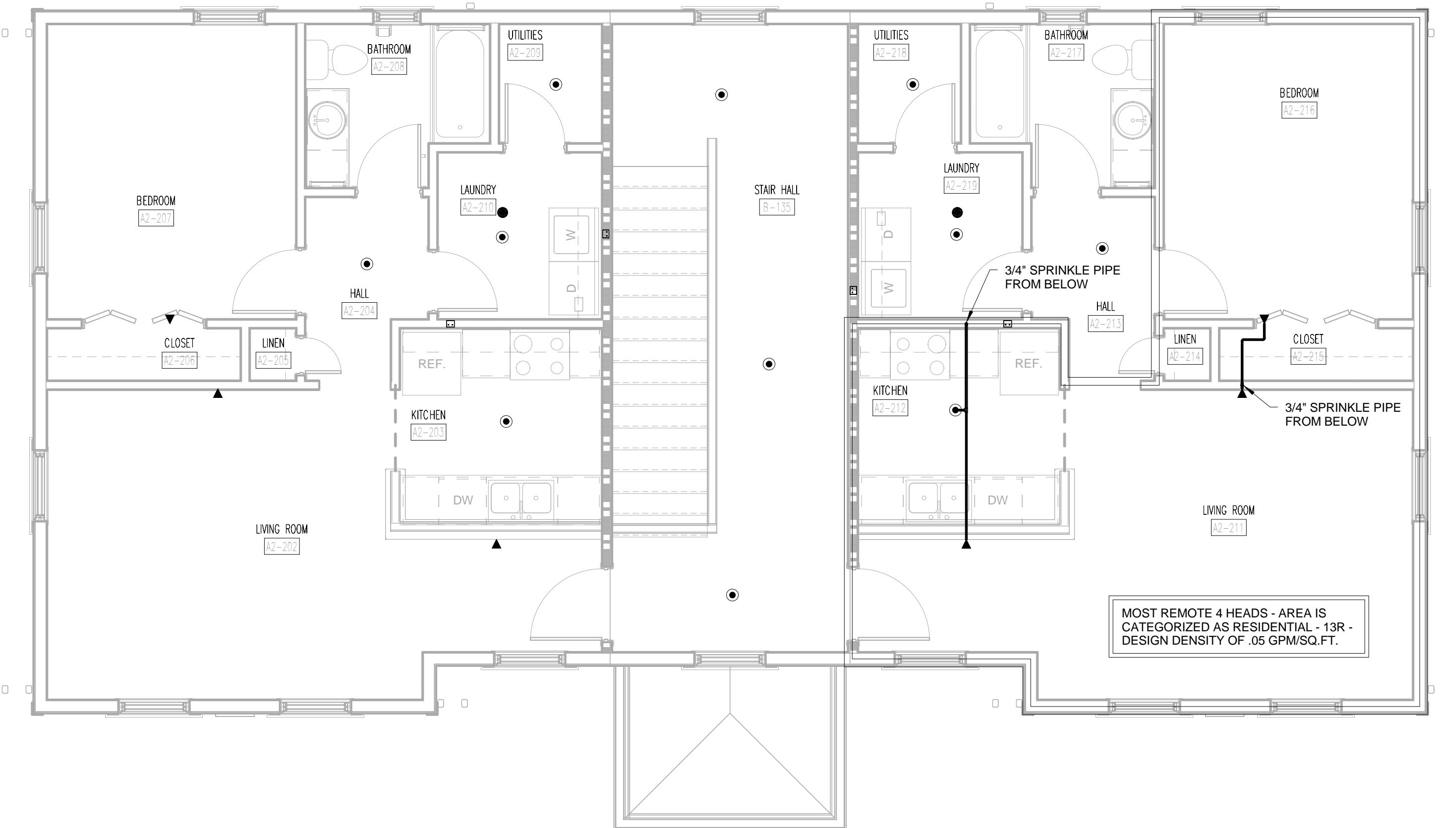
TYPE A2 SECOND FLOOR FIRE PROTECTION PLAN 1/4" = 1'-0"
