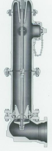
☐ REVERSIBLE, COMPRESSION TYPE MAIN VALVE - closes with pressure for positive seal. Rubber material has long service life, yet is reversible providing a convenient spare in place.
