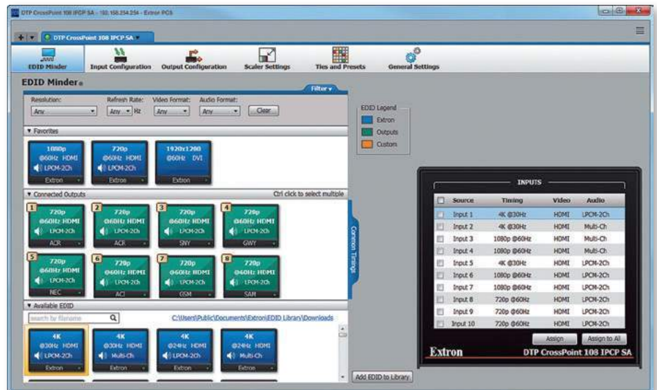
The intuitive user interface makes it easy to independently apply EDID settings to each input, allowing the user to select from EDID captured from connected output devices, factory default EDID, or custom EDID uploaded to the unit.
