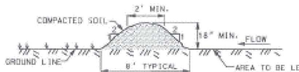
EXCEPT AT DRIVES TEMPORARY DIVERSION DIKE
