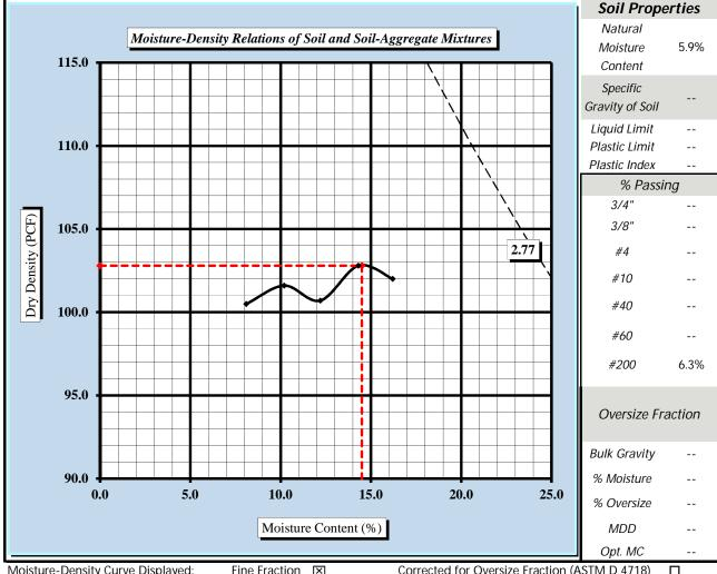
Moisture-Density Curve Displayed: Fine Fraction ☑ Corrected for Oversize Fraction (ASTM D 4718) ☐
