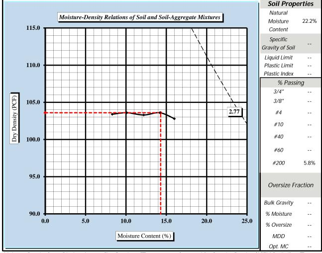
Moisture-Density Curve Displayed: Corrected for Oversize Fraction (ASTM D 4718) Fine Fraction 🗵 Sieve Size used to separate the Oversize Fraction: #4 Sieve 区 3/8 inch Sieve □ 3/4 inch Sieve □ Mechanical Rammer Manual Rammer Moist Preparation □ Dry Preparation **区** References / Comments / Deviations:
