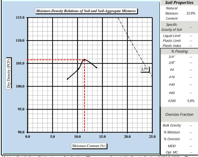
Moisture-Density Curve Displayed: Corrected for Oversize Fraction (ASTM D 4718) Fine Fraction 🗵 Sieve Size used to separate the Oversize Fraction: #4 Sieve 区 3/8 inch Sieve □ 3/4 inch Sieve □ Mechanical Rammer Manual Rammer Moist Preparation □ Dry Preparation **区**
