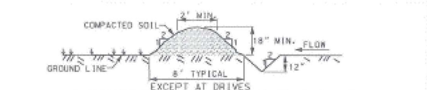
EXCEPT AT DRIVES TEMPORARY DIVERSION DIKE WITH DITCH THE PAY ITEM SHALL BE: TEMPORARY DIVERSION DIKE WITH DITCH.....L.F.
