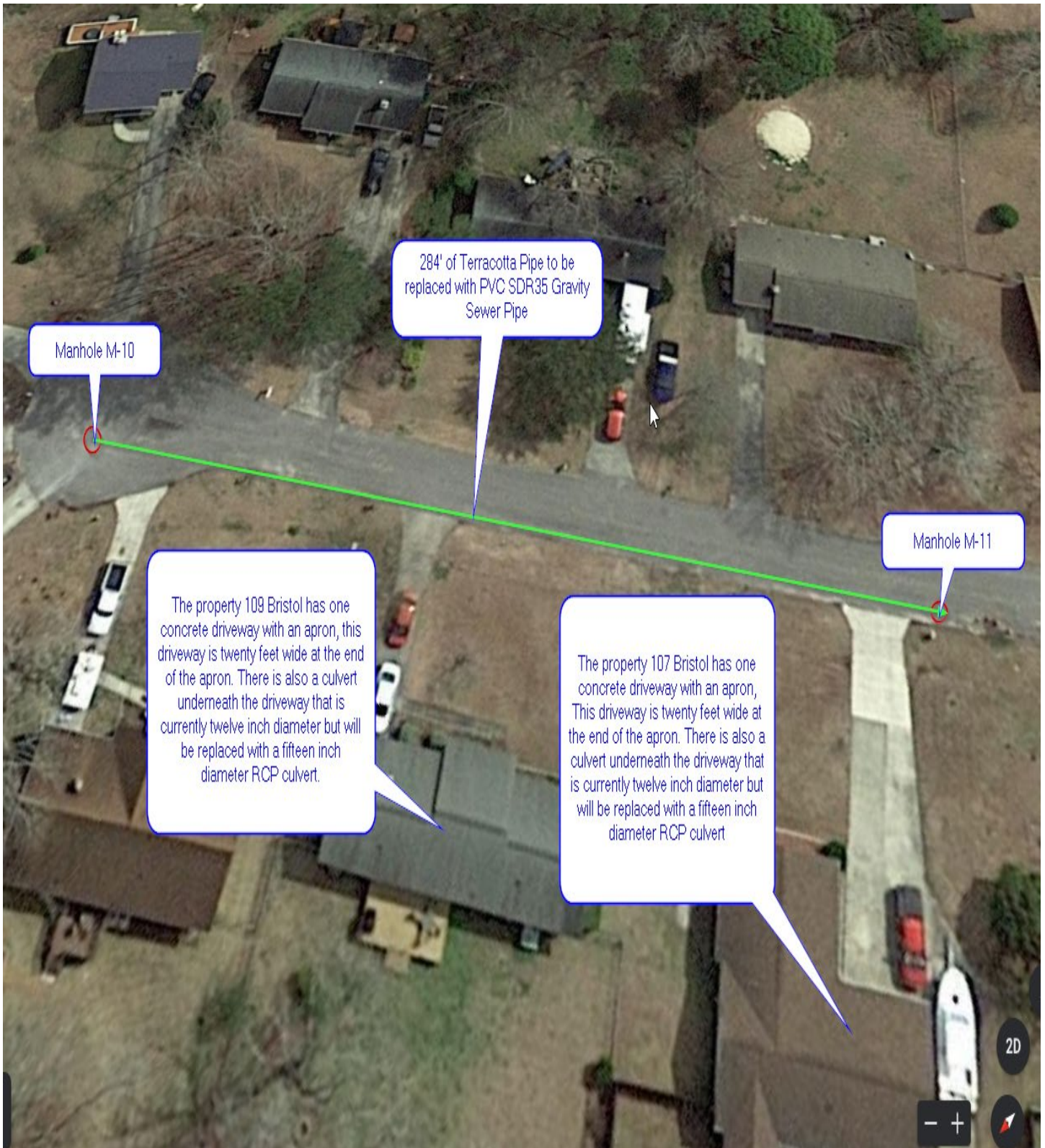
Figure 2: Driveways and culverts between Manholes M-11 and M-10
