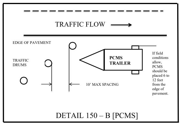
When not in use, the PCMS shall be removed from the roadway, unless protected by positive barrier protection. If the PCMS is protected by positive barrier protection, the sign panel shall be turned away from traffic when not in use.
