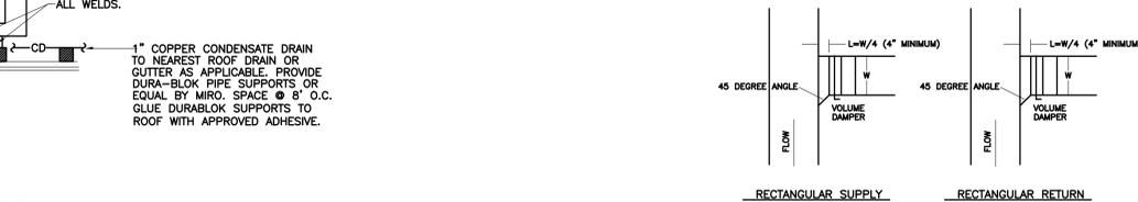
**DUCT BRANCH FITTING DETAIL**
