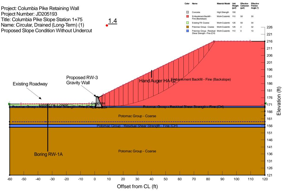
Note: Data point is randomly placed to show factor of safety value only and does not represent the true center of the critical slip surface. Actual coordinates of the center of critical slip surface are: (2.5072077, 264.26104) ft
