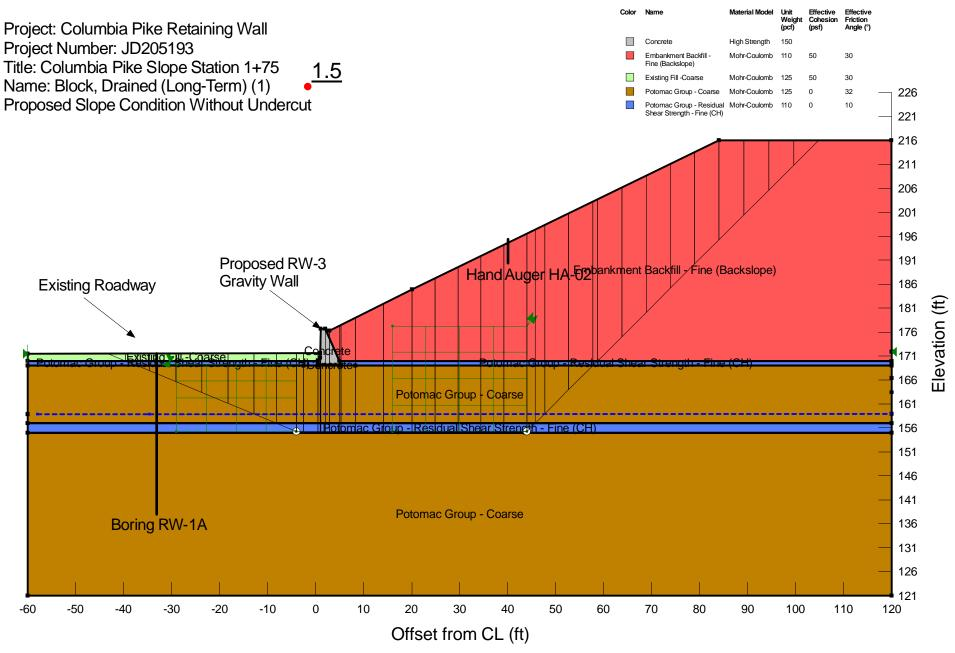
Note: Data point is randomly placed to show factor of safety value only and does not represent the true center of the critical slip surface. Actual coordinates of the center of critical slip surface are: (20.721057, 227.18265) ft
