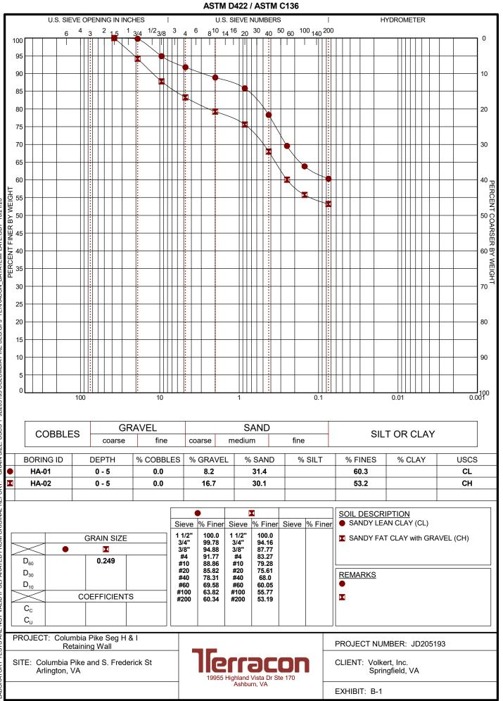
GRAIN SIZE: USCS 1 JD205193 COLUMBIA PIKE SEG.GPJ TERRACON\_DATATEMPLATE.GDT 10/21/20 REPORT. ABORATORY TESTS ARE NOT VALID IF SEPARATED FROM ORIGINAL **GRAIN SIZE DISTRIBUTION**
