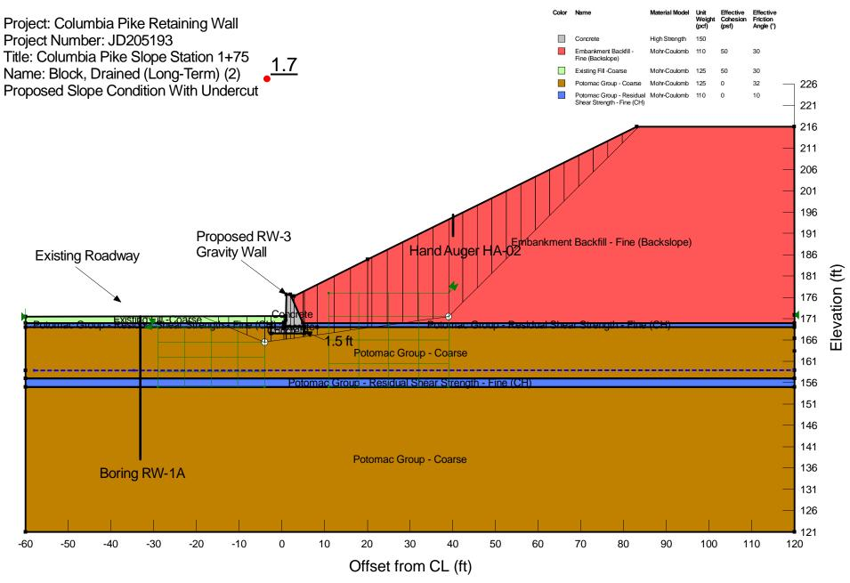
Note: Data point is randomly placed to show factor of safety value only and does not represent the true center of the critical slip surface. Actual coordinates of the center of critical slip surface are: (17.928358, 227.13122) ft
