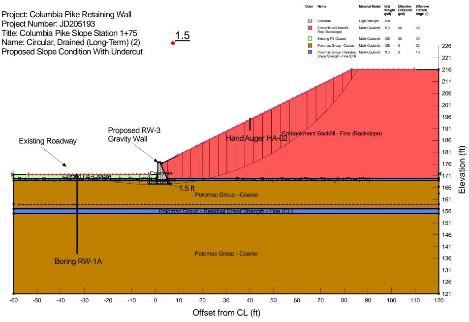
Note: Data point is randomly placed to show factor of safety value only and does not represent the true center of the critical slip surface. Actual coordinates of the center of critical slip surface are: (-0.72491392, 268.02529) ft
