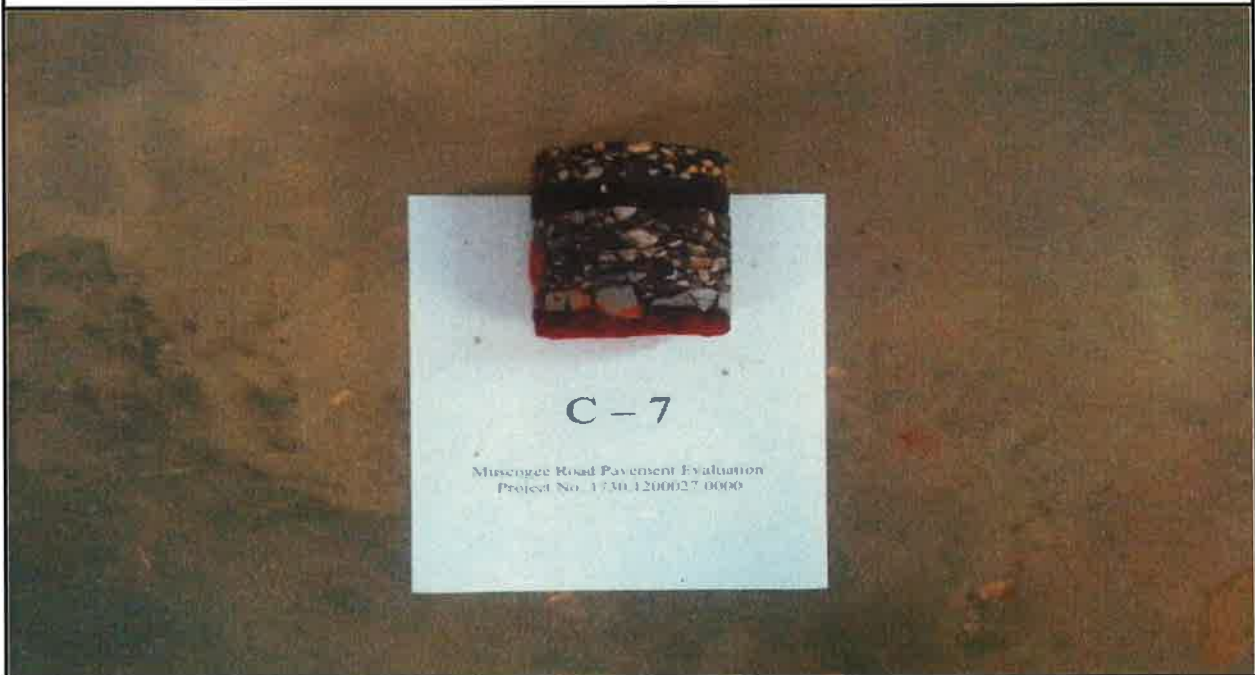
Photo 14: Pavement core C-7.
