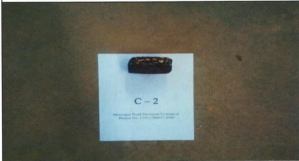
Photo 4: Pavement core C - 2.
