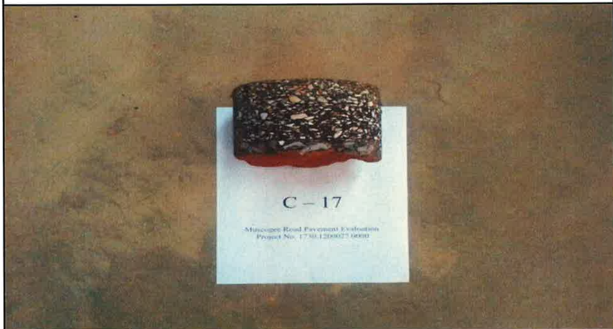
Photo 34 : Pavement core C-17.
