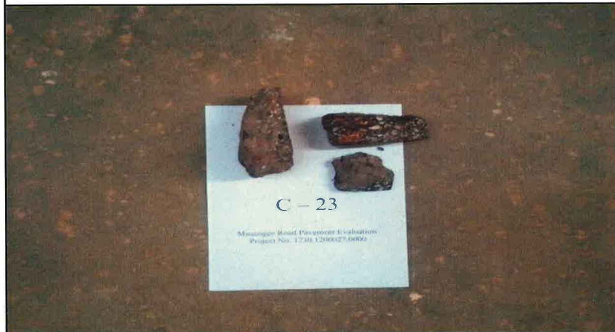
Photo 46: Pavement core C-23.
