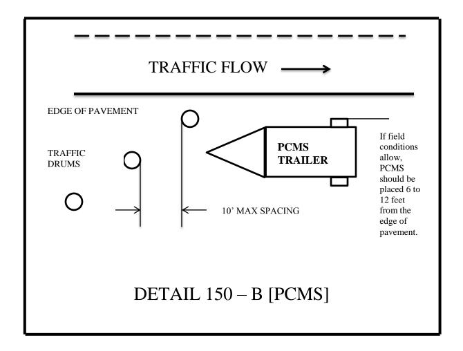
When not in use, the PCMS shall be removed from the roadway, unless protected by positive barrier protection. If the PCMS is protected by positive barrier protection, the sign panel shall be turned away from traffic when not in use.
