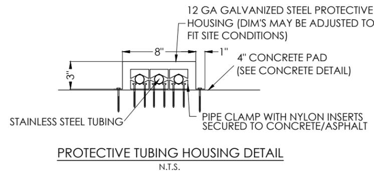
PROTECTIVE TUBING HOUSING DETAIL
