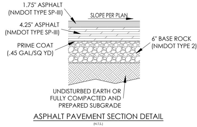
ASPHALT PAVEMENT SECTION DETAIL
