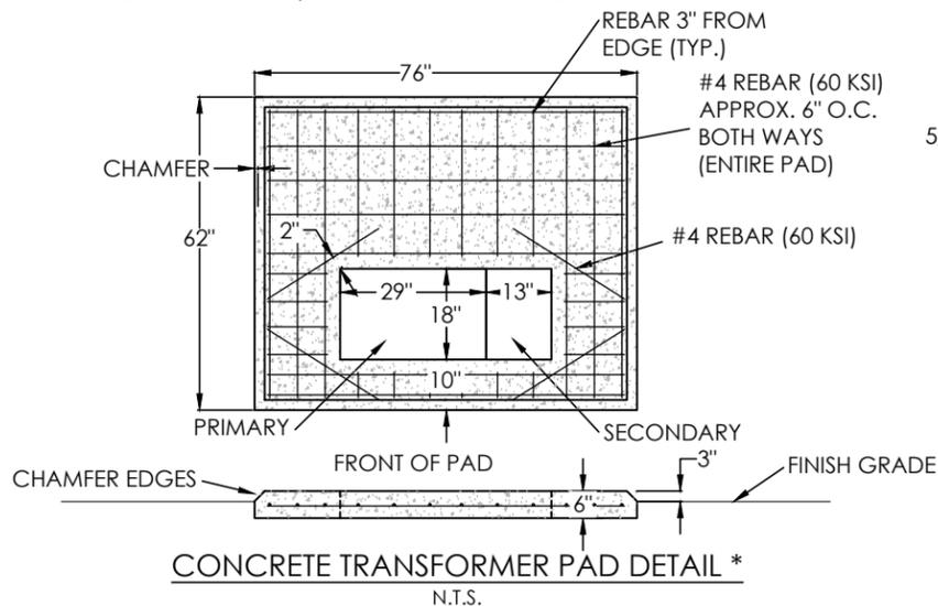
**CONCRETE TRANSFORMER PAD DETAIL \***
