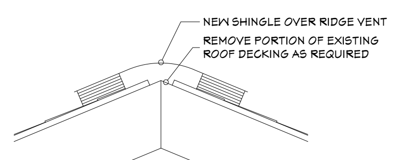
Ridge Vent Detail NOT TO SCALE
