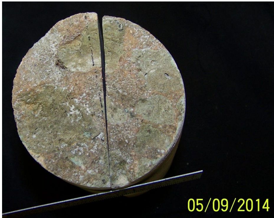
Photo 3 – Sample 3A – end view, note surface erosion.
