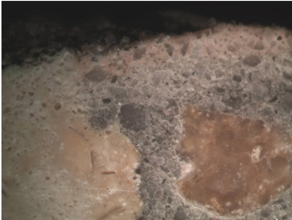
Photo 7 – Sample 3A – variation in paste coloration, tan near surface to darker gray between coarse aggregate.
