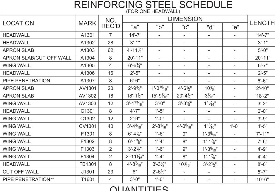
(FOR ONE HEADWALL) **UNIT** QTY. ITEM CONC. FOR STRUCTURES CLASS 4000 (CULVERT) CY 8.6 REINFORCING STEEL FOR STRUCTURES (ROADWAY) LB 1,252
