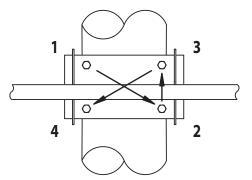
Using supplied breaker bar, 1<sup>1</sup>/<sub>16</sub> in socket, extension, and wrench, tighten each nut until orange extrusion appears from at least three bumps.
