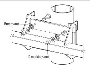
Snug all nuts. Using supplied 1<sup>1</sup>/<sub>16</sub> in wrench, tighten each nut until plates are in firm contact. Follow tightening sequence shown.
