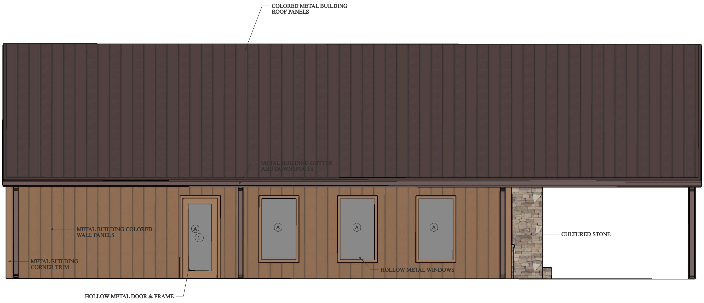
LEFT SIDE ELEVATION SCALE 1/4" = 1'-0"
