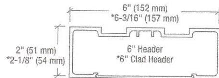
CRL Single Door Headers are fabricated to hold our overhead concealed door closers. Headers are carried in three stock sizes, and custom sizes can be special ordered. Headers are supplied with an Aluminum Mounting Clip for mounting the Header on the opposite side of the door closer. The door closer contains the mounting clip for that side of the Header. Snap-In cover plates allow for easy installation of the closer. **NOTE:** Clad and anodized Headers differ in size.
