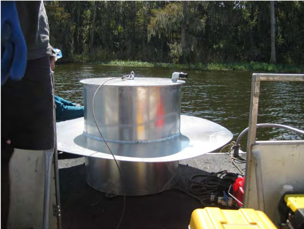
Figure 2-3. Typical Seepage Meter Used in Lake Jesup.
